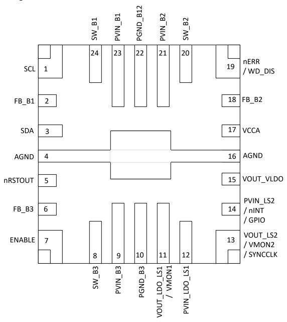
Figure 5-1. Package 24-Pin VQFN-HR Top View
