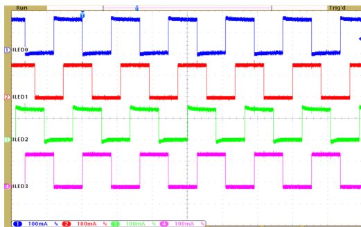
Figure 8-3. LED String Currents Showing Phase Shift PWM Operation
