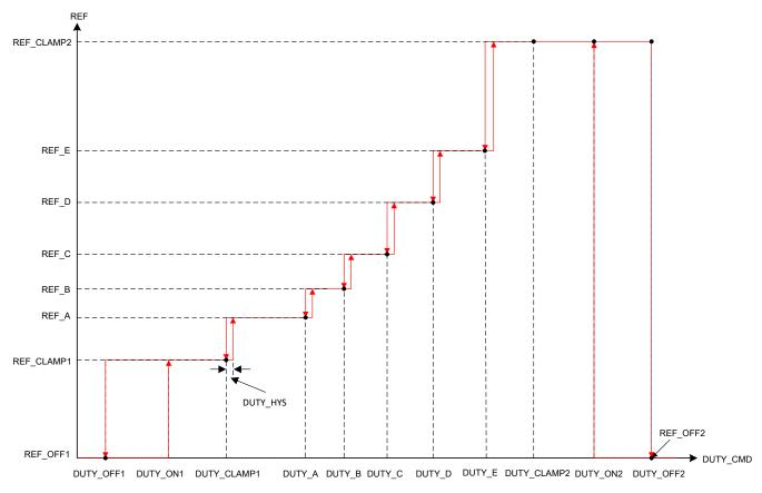
Figure 7-12. Staircase Control Profiles
