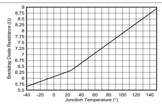
Figure 6-3. Bootstrap Diode Resistance over **Junction Temperature**
