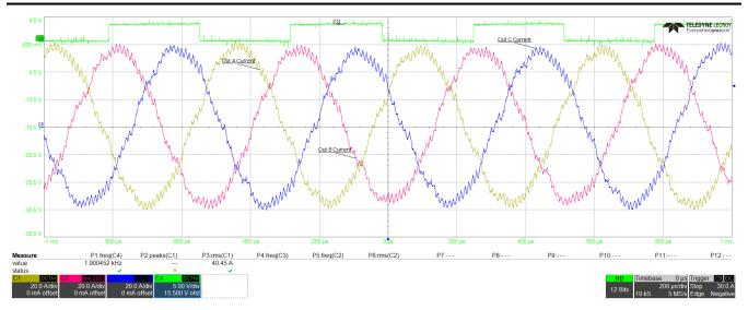
Figure 8-6. Phase currents at 1.8 kHz motor speed
