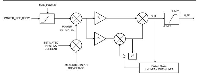
Figure 7-32. Closed Loop Power Control
