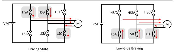
Figure 7-43. Low-Side Braking
