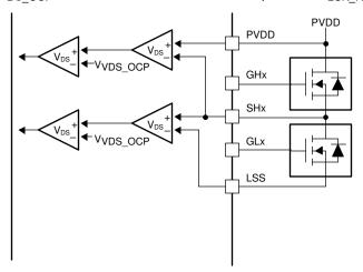
Figure 7-49. MCF8329A VDS Monitors
