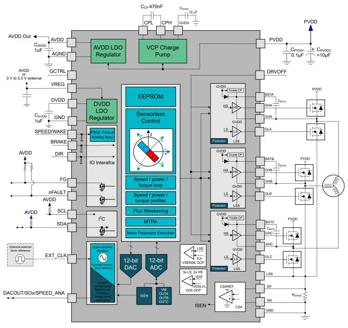
Figure 7-1. MCF8329A Functional Block Diagram
