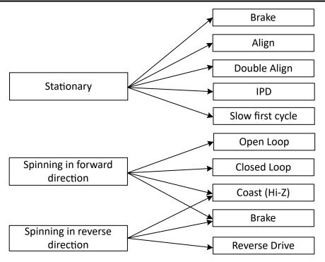
Figure 7-18. Starting the motor under different initial conditions
