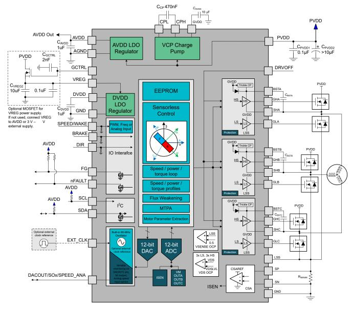
Figure 8-1. Typical Schematic of MCF8329A
