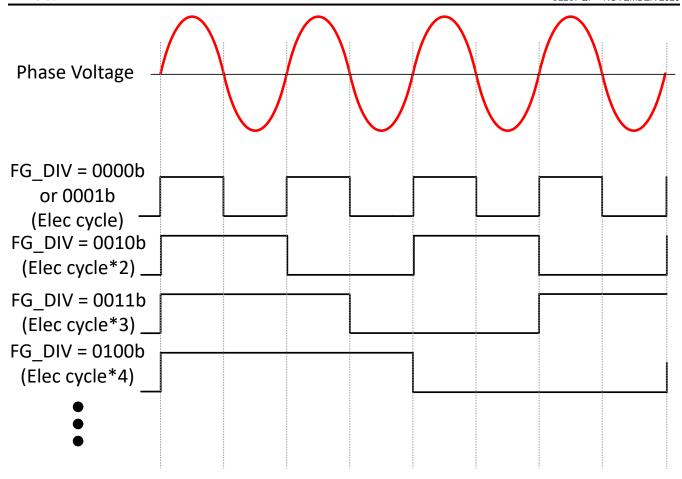
Figure 7-44. FG Frequency Divider
