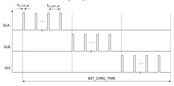
Figure 7-17. Bootstrap Capacitor Precharging at Start up
