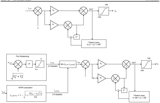
Figure 7-34. Flux Weakening Control
