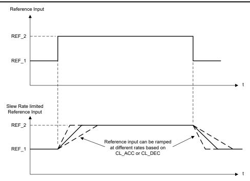
Figure 7-28. Closed Loop Acceleration/Deceleration Slew Rate
