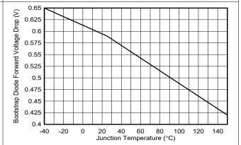
Figure 6-4. Bootstrap Diode Forward Voltage Drop over Junction Temperature
