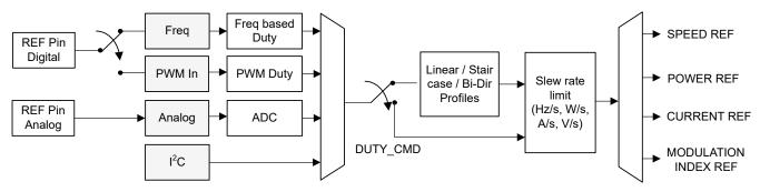
Figure 7-7. Multiplexing the Reference Input Command
