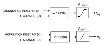
Figure 7-33. Open Loop Voltage Control
