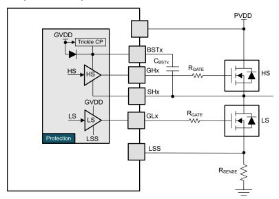
Figure 8-2. Gate driver outputs with series resistors
