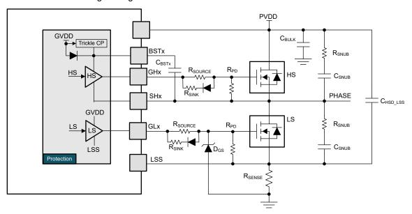
Figure 8-4. Optional external power stage components
