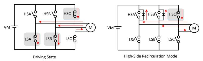
Figure 7-42. High-Side Recirculation
