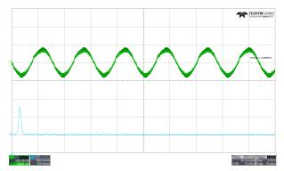
Figure 8-10. Phase current and FFT - Dead time compensation enabled
