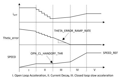
Figure 7-25. Control Sequence in Open to Closed Loop Transition
