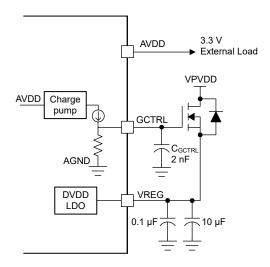
Figure 7-6. External MOSFET Voltage Regulator for VREG
