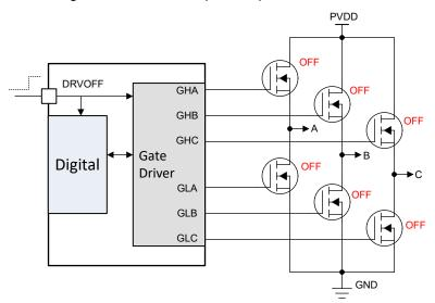
Figure 7-50. DRVOFF Gate Driver Output State
