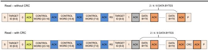
CRC includes {TARGET ID,0}, CONTROL WORD[23:0], {TARGET ID,1}, DATA BYTES
