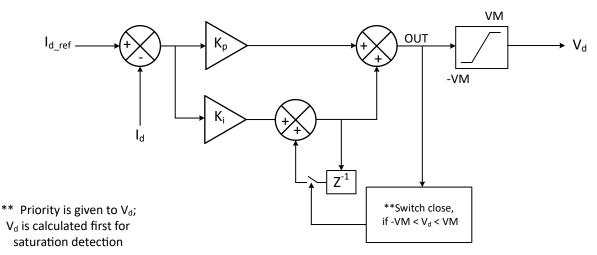
Figure 7-30. I<sub>d</sub> Current PI Control
