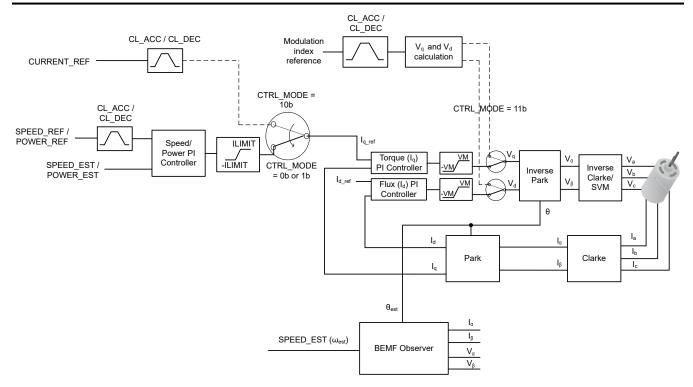
Figure 7-27. Closed Loop FOC Control
