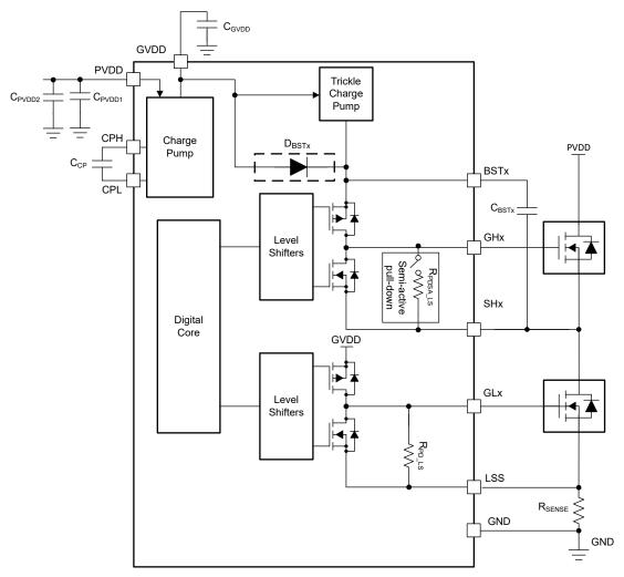
Figure 7-2. Gate Driver Block Diagram
