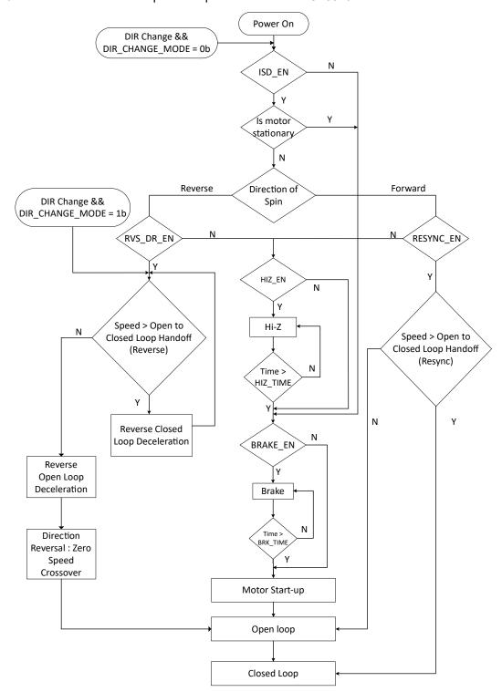
Figure 7-19. Motor Starting-up Flow
