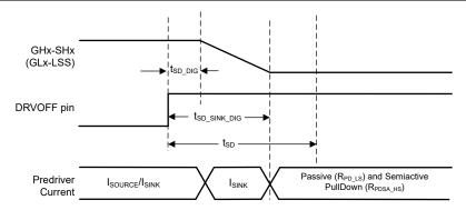
Figure 7-51. Gate Driver Shutdown Sequence
