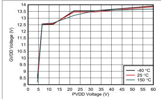
Figure 6-1. GVDD Voltage over PVDD Voltage
