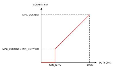
Figure 7-16. Current Input Transfer Function
