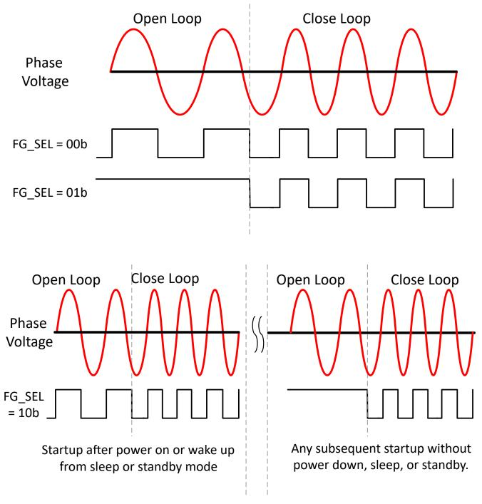
Figure 7-45. FG Behavior During Open Loop
