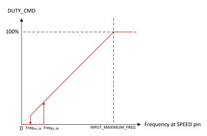
Figure 7-10. Frequency-Mode Motor Control
