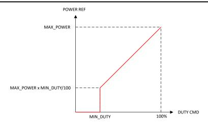
Figure 7-15. Power Input Transfer Function
