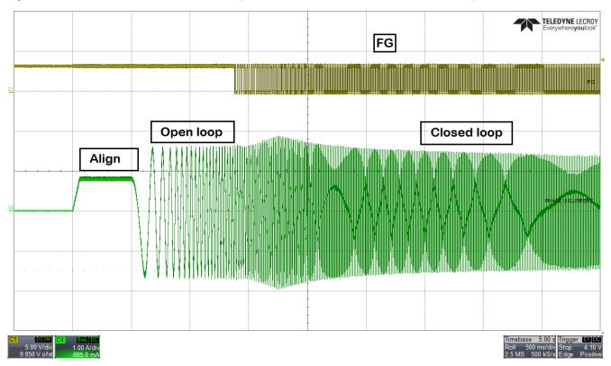
Figure 8-5. Motor Startup - FG and Phase current
