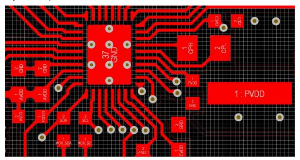
Figure 10-1. Layout example of MCF8329A device
