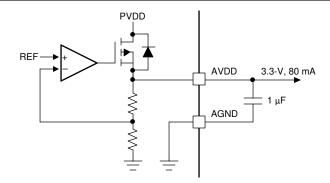
Figure 7-3. AVDD Linear Regulator Block Diagram
