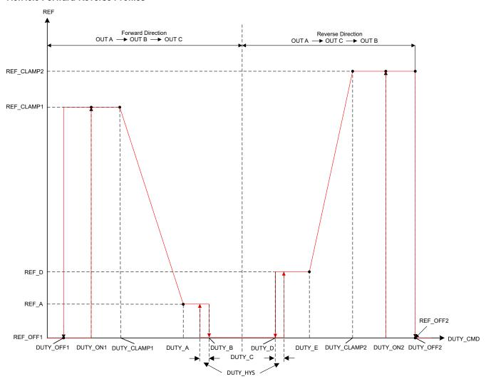
Figure 7-13. Forward Reverse Control Profiles
