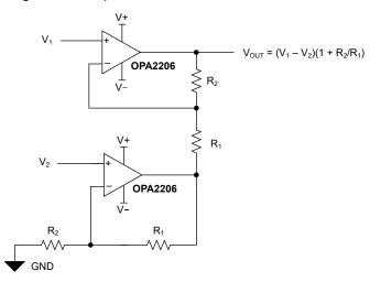
Figure 8-4. OPA2206 Configured as a Two Op Amp, Discrete Instrumentation Amplifier
