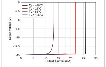
Figure 5-29. Output Voltage Swing vs Output Sourcing Current
