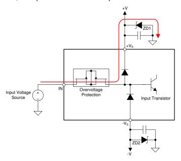
Figure 7-1. OPAx206 Input Overvoltage Current Path
