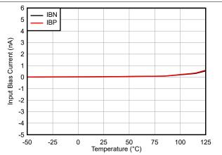
Figure 7-7. OPAx206 Super-Beta Input Bias Current
