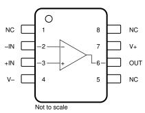
Figure 4-1. OPA206: D Package, 8-Pin SOIC (Top View)
