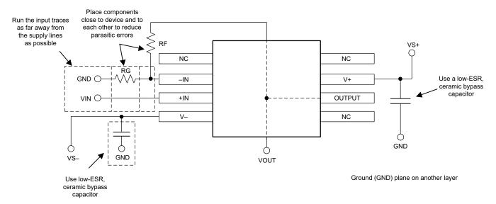
Figure 8-7. Operational Amplifier Board Layout for Noninverting Configuration
