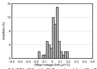
Figure 7-5. OPAx206 e-trim™ Operational Amplifier Drift
