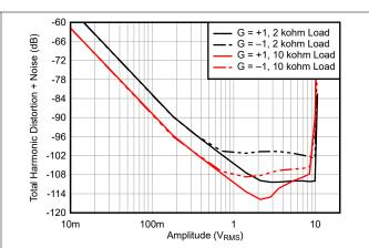
Figure 5-25. Total Harmonic Distortion + Noise Ratio vs Frequency
