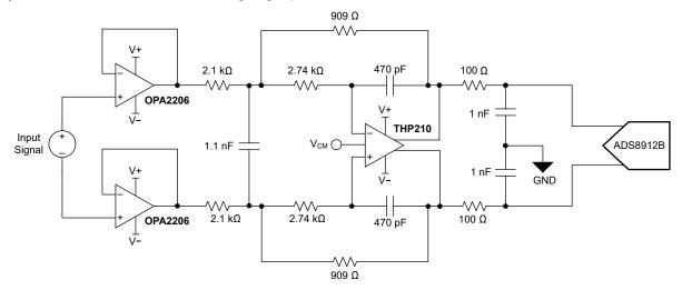
Figure 8-5. OPA2206 Configured as an Input-Signal-Chain Buffer
