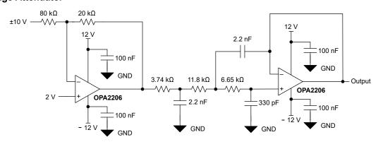
Figure 8-1. OPA2206 Configured as a Voltage Attenuator
