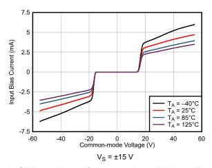
Figure 7-2. OPAx206 Input Current vs Input Voltage ( $V_S = \pm 15 \text{ V}$ )
