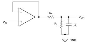
Figure 7-1. Improving Capacitive Load Drive
