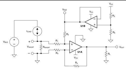
Figure 7-2. Bidirectional Current-Sensing Schematic
