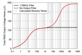
Figure 7-15. Transimpedance Amplifier RC-Filter Noise Comparison
