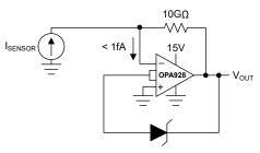
Figure 7-16. Improved Diode Limiter
