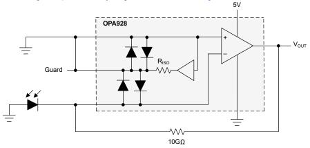
Figure 7-4. Single-Supply Transimpedance Amplifier With Grounded Guard Pin
