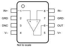
Figure 4-1. D Package, 8-Pin SOIC (Top View)
