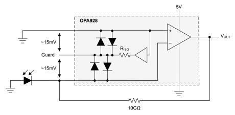
Figure 7-3. Single-Supply Transimpedance Amplifier
