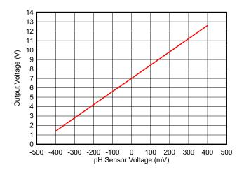
Figure 7-9. Single Supply, pH-Probe Sensor Transfer Function
