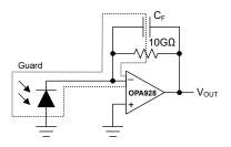
Figure 7-10. Simplified Photodiode Transimpedance Amplifier With the OPA928
