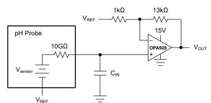
Figure 7-8. pH Probe Simplified Model
