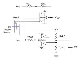
Figure 7-7. High Impedance pH Probe Amplifier Circuit
