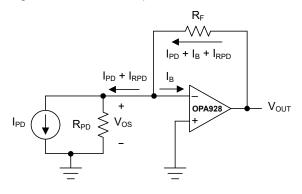
$V_{OUT} = I_{PD}R_F + I_BR_F + V_{OS}(1+R_F/R_{PD})$
