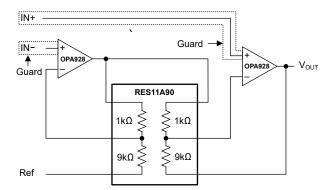
Figure 7-19. Two Op Amp Instrumentation Amplifier
