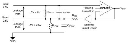
Figure 7-2. Driving the Guard, External Guard Driver
