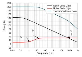
Figure 7-13. Transimpedance Amplifier Noise Gain
