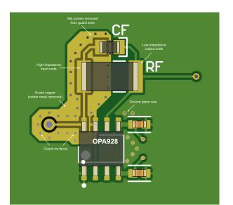
Figure 7-22. Layout Example: Inverting Configuration
