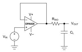
Figure 6-1. Extending Capacitive Load Drive With the OPA928
