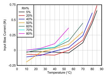
Figure 7-6. Input Bias Current vs Temperature at Various Levels of Relative Humidity
