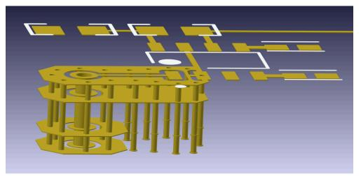
Figure 7-23. Layout Example: Three-Dimensional Guard (4-Layer PCB)
