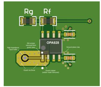
Figure 7-21. Layout Example: Noninverting Configuration
