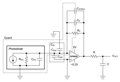
Figure 7-11. Transimpedance Photodiode Application
