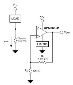
Figure 8-1. OPAx992-Q1 in a Low-Side, Current-Sensing Application
