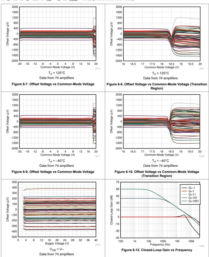
Figure 6-11. Offset Voltage vs Power Supply
