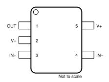
Figure 5-1. OPA992-Q1 DBV Package, 5-Pin SOT-23 (Top View)
