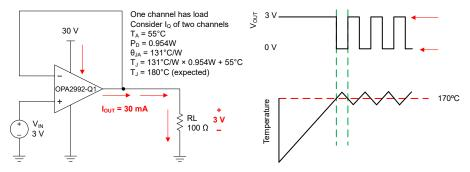
Figure 7-4. Thermal Protection
