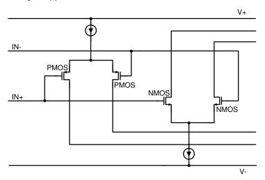
Figure 7-8. Rail-to-Rail Input Stage
