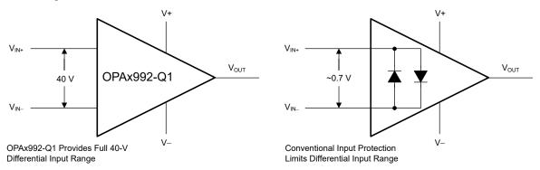
Figure 7-1. OPAx992-Q1 Input Protection Does Not Limit Differential Input Capability
