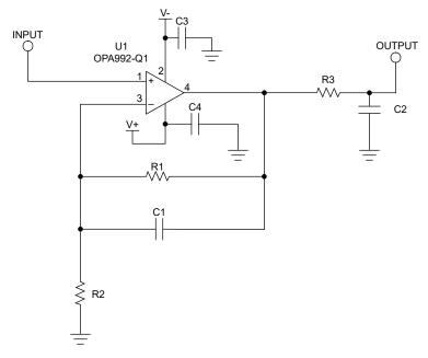
Figure 8-3. Schematic for Noninverting Configuration Layout Example
