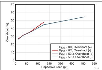
Figure 7-6. Small-Signal Overshoot vs Capacitive Load (20-mV<sub>pp</sub> Output Step, G = -1)
