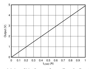
Figure 8-2. Low-Side, Current-Sense, Transfer Function
