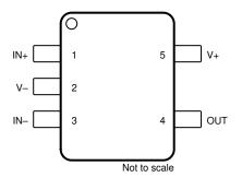
Figure 5-2. OPA992-Q1 DCK Package, 5-Pin SC70 (Top View)
