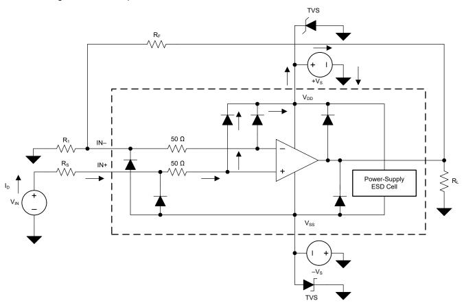
Figure 7-10. Equivalent Internal ESD Circuitry Relative to a Typical Circuit Application
