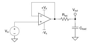
Figure 7-7. Extending Capacitive Load Drive With the OPA992-Q1
