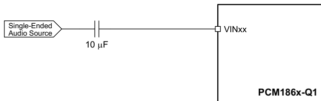
Figure 60. Analog Input Circuit for Single-Ended Input Applications
