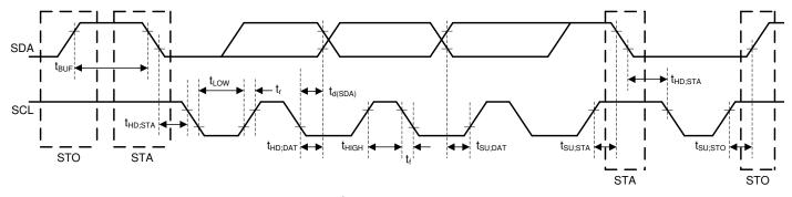
Figure 6-1. I<sup>2</sup>C Interface Timing Diagram
