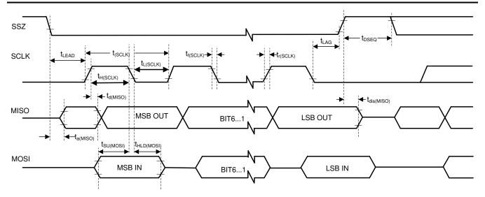
Figure 6-2. SPI Interface Timing Diagram
