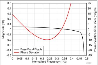
Figure 7-50. Ultra-Low-Latency Decimation Filter Pass-Band Ripple and Phase Deviation
