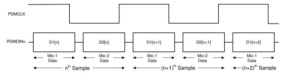
Figure 7-65. Digital PDM Microphone Protocol Timing Diagram
