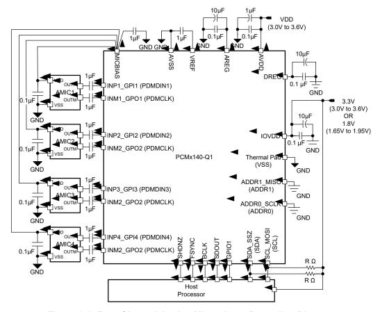
Figure 9-1. Four-Channel Analog Microphone Recording Diagram
