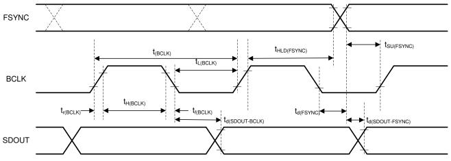
Figure 6-3. TDM (With BCLK\_POL = 1), I<sup>2</sup>S, and LJ Interface Timing Diagram
