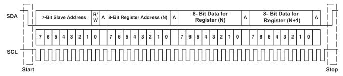
Figure 7-66. Typical I<sup>2</sup>C Sequence
