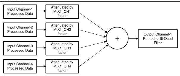
Figure 7-18. Programmable Digital Mixer Block Diagram
