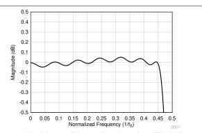
Figure 7-22. Linear Phase Decimation Filter Pass-Band Ripple
