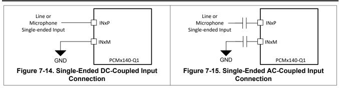
The device allows for flexibility in choosing the typical input impedance on INxP or INxM from 2.5 k $\Omega$  (default), 10 k $\Omega$ , and 20 k $\Omega$  based on the input source impedance. The higher input impedance results in slightly higher noise or lower dynamic range. Table 7-9 lists the configuration register settings for the input impedance for the record channel.
