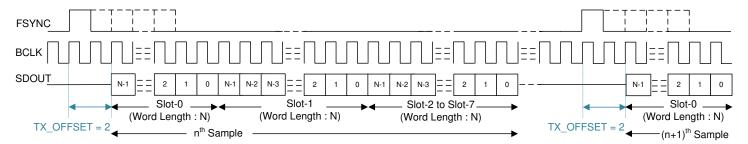
Figure 7-2. TDM Mode Protocol Timing (TX\_OFFSET = 2)
