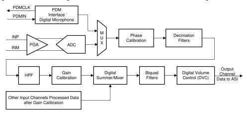
Figure 7-16. Signal-Chain Processing Flowchart
