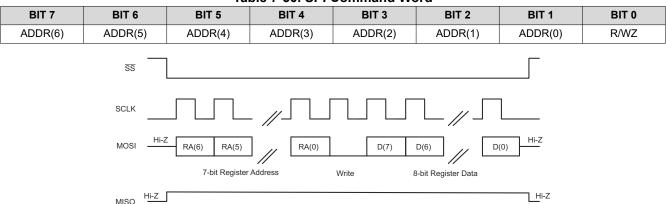
Figure 7-71. SPI Single-Byte Write Transfer
