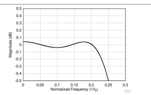
Figure 7-34. Linear Phase Decimation Filter Pass-Band Ripple
