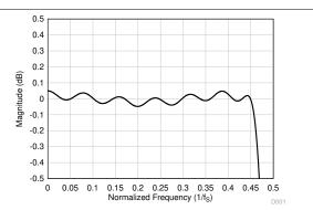
Figure 7-30. Linear Phase Decimation Filter Pass-Band Ripple
