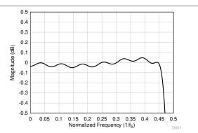
Figure 7-26. Linear Phase Decimation Filter Pass-Band Ripple
