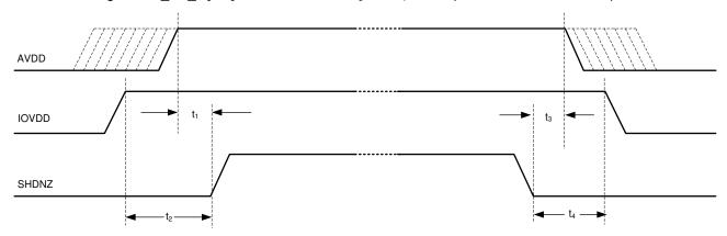
Figure 9-5. Power-Supply Sequencing Requirement Timing Diagram
