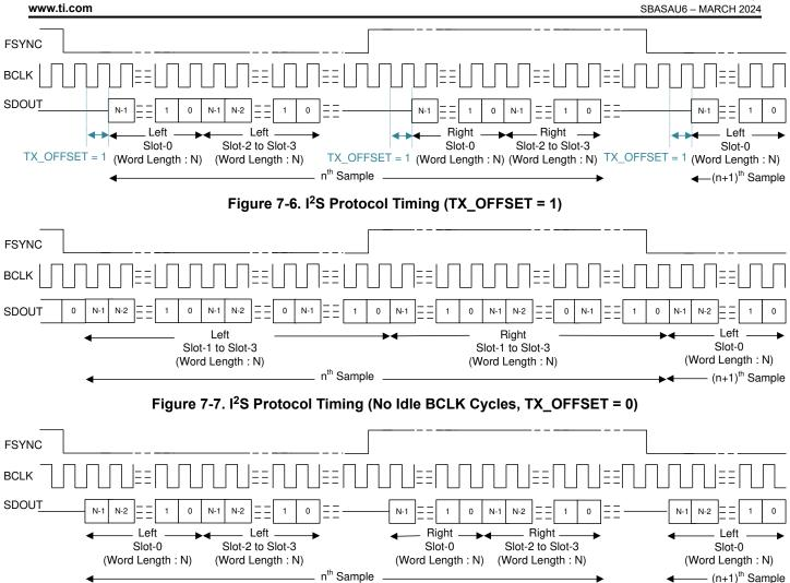
Figure 7-8. I<sup>2</sup>S Protocol Timing (TX\_OFFSET = 0 and BCLK\_POL = 1)
