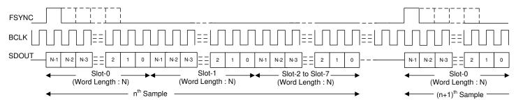
Figure 7-4. TDM Mode Protocol Timing (TX\_OFFSET = 0 and BCLK\_POL = 1)
