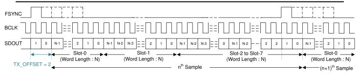
Figure 7-3. TDM Mode Protocol Timing (No Idle BCLK Cycles, TX\_OFFSET = 2)
