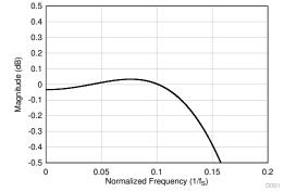
Figure 7-36. Linear Phase Decimation Filter Pass-Band Ripple
