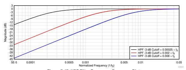
Figure 7-17. HPF Filter Frequency Response Plot
