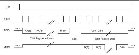
Figure 7-72. SPI Single-Byte Read Transfer
