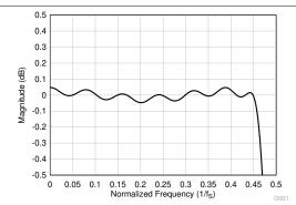
Figure 7-24. Linear Phase Decimation Filter Pass-Band Ripple
