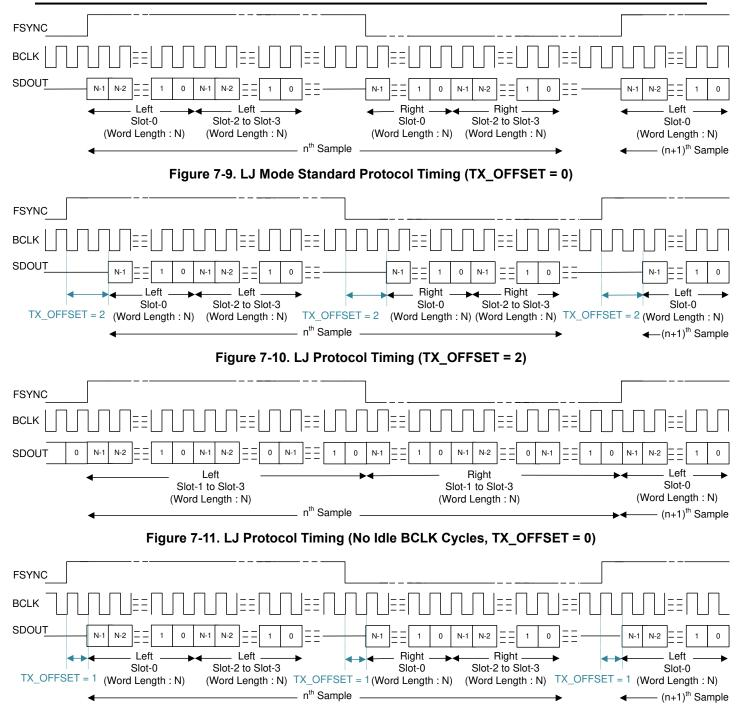
Figure 7-12. LJ Protocol Timing (TX\_OFFSET = 1 and BCLK\_POL = 1)
