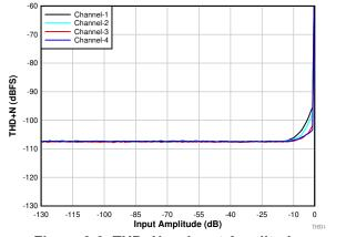
Figure 9-3. THD+N vs Input Amplitude
