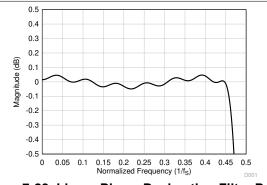
Figure 7-28. Linear Phase Decimation Filter Pass-Band Ripple
