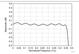
Figure 7-20. Linear Phase Decimation Filter Pass-Band Ripple
