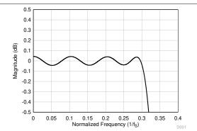
Figure 7-32. Linear Phase Decimation Filter Pass-Band Ripple
