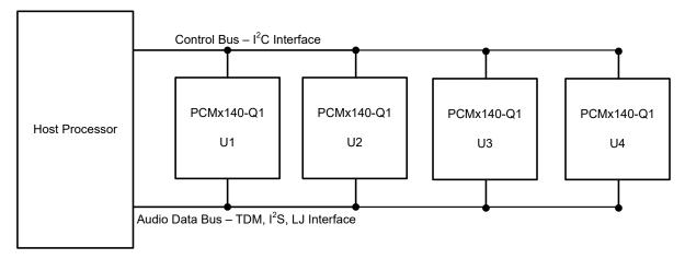
Figure 7-13. Multiple PCM3140-Q1 Devices With Shared Control and Audio Data Buses
