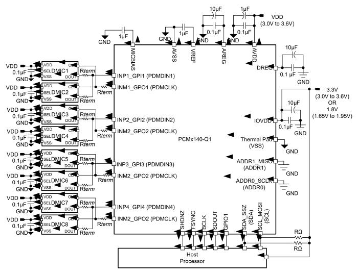
Figure 9-4. Eight-Channel Digital PDM Microphone Recording Diagram
