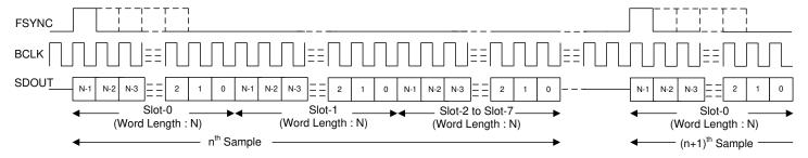
Figure 7-1. TDM Mode Standard Protocol Timing (TX OFFSET = 0)
