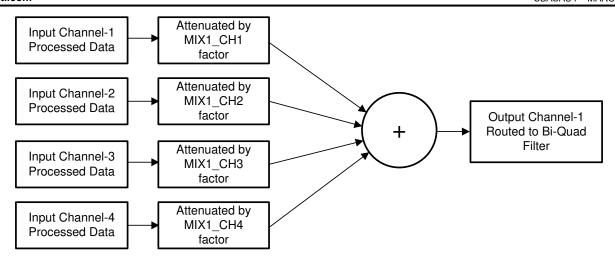
Figure 7-18. Programmable Digital Mixer Block Diagram
