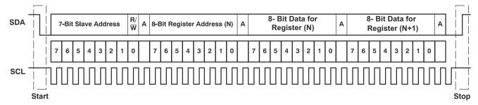
Figure 7-66. Typical I<sup>2</sup>C Sequence
