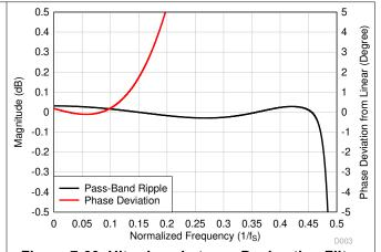
Figure 7-59. Ultra-Low-Latency Decimation Filter Magnitude Response
