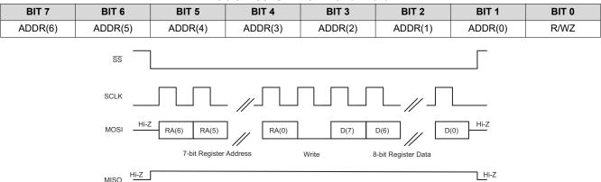
Figure 7-71. SPI Single-Byte Write Transfer
