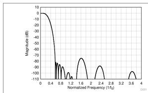
Figure 7-35. Linear Phase Decimation Filter
