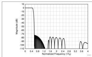
Figure 7-23. Linear Phase Decimation Filter
