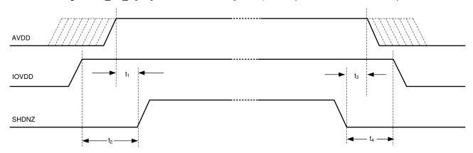
Figure 9-7. Power-Supply Sequencing Requirement Timing Diagram
