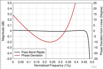
Figure 7-51. Ultra-Low-Latency Decimation Filter Magnitude Response
