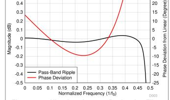
Figure 7-53. Ultra-Low-Latency Decimation Filter Magnitude Response
