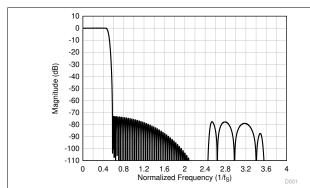
Figure 7-21. Linear Phase Decimation Filter Magnitude Response
