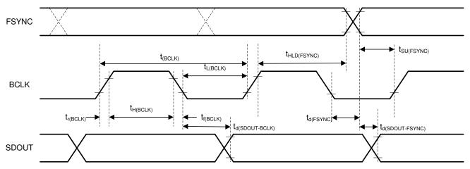
Figure 6-3. TDM (With BCLK\_POL = 1), I<sup>2</sup>S, and LJ Interface Timing Diagram
