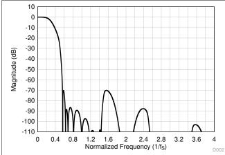
Figure 7-61. Ultra-Low-Latency Decimation Filter Magnitude Response
