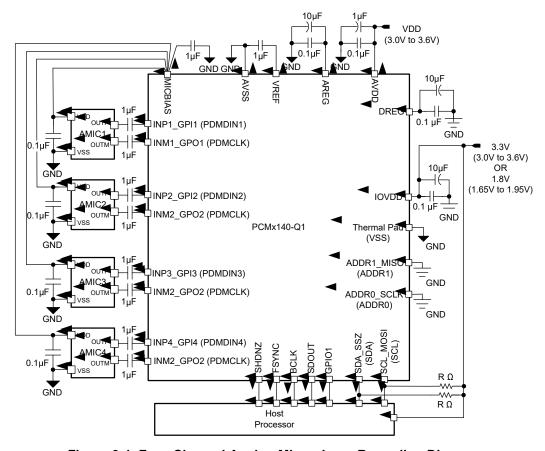
Figure 9-1. Four-Channel Analog Microphone Recording Diagram
