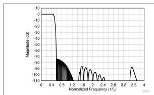
Figure 7-29. Linear Phase Decimation Filter
