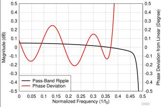
Figure 7-37. Low-Latency Decimation Filter Magnitude Response
