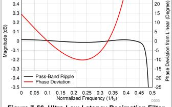
Figure 7-55. Ultra-Low-Latency Decimation Filter Magnitude Response
