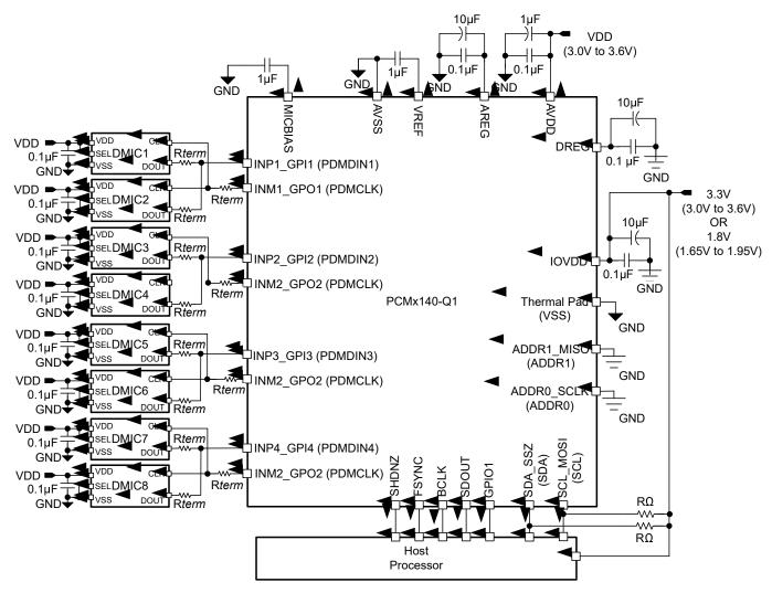
Figure 9-6. Eight-Channel Digital PDM Microphone Recording Diagram
