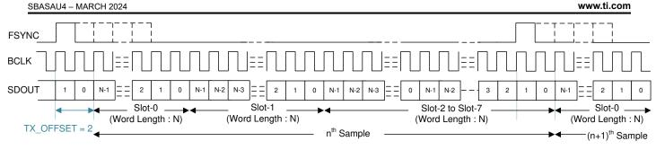
Figure 7-3. TDM Mode Protocol Timing (No Idle BCLK Cycles, TX\_OFFSET = 2)
