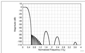
Figure 7-33. Linear Phase Decimation Filter Magnitude Response
