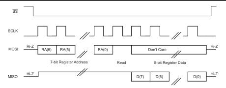
Figure 7-72. SPI Single-Byte Read Transfer
