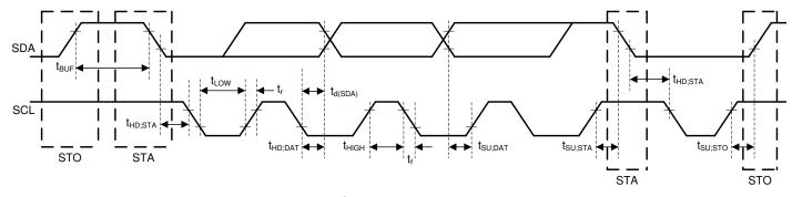
Figure 6-1. I<sup>2</sup>C Interface Timing Diagram
