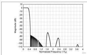
Figure 7-31. Linear Phase Decimation Filter Magnitude Response
