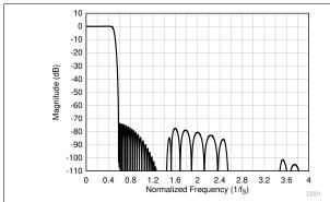
Figure 7-25. Linear Phase Decimation Filter Magnitude Response
