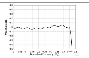
Figure 7-26. Linear Phase Decimation Filter Pass-Band Ripple
