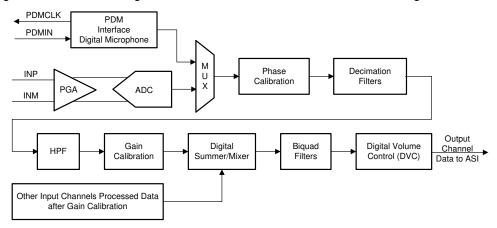
Figure 7-16. Signal-Chain Processing Flowchart
