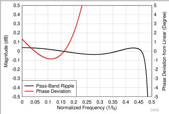
Figure 6-57. Ultra-Low-Latency Decimation Filter Magnitude Response
