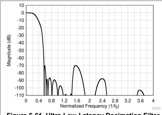
Figure 6-61. Ultra-Low-Latency Decimation Filter Magnitude Response
