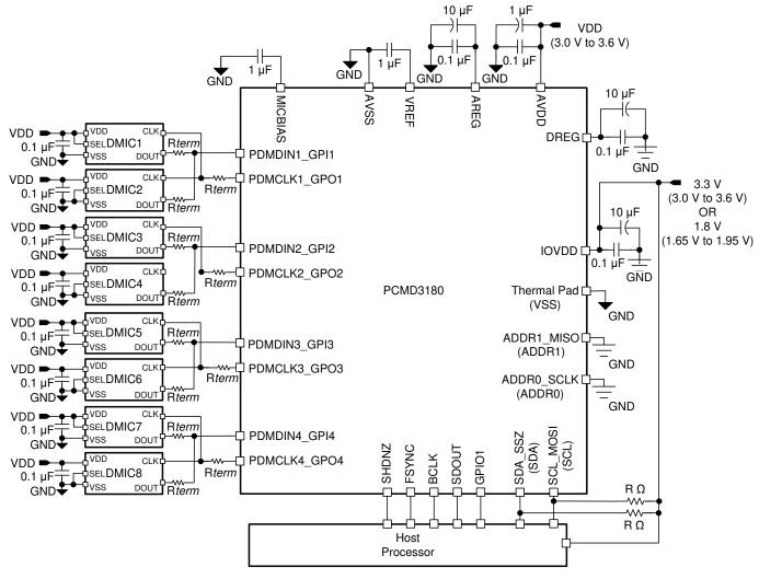
Figure 8-1. Eight-Channel Digital PDM Microphone Recording Diagram
