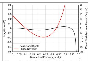
Figure 6-53. Ultra-Low-Latency Decimation Filter Magnitude Response
