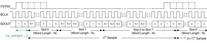
Figure 6-3. TDM Mode Protocol Timing (No Idle BCLK Cycles, TX\_OFFSET = 2)
