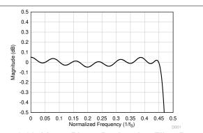
Figure 6-30. Linear Phase Decimation Filter Pass-**Band Ripple**
