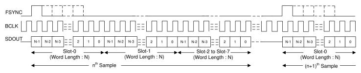
Figure 6-4. TDM Mode Protocol Timing (TX\_OFFSET = 0 and BCLK\_POL = 1)
