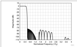
Figure 6-25. Linear Phase Decimation Filter Magnitude Response
