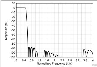
Figure 6-49. Ultra-Low-Latency Decimation Filter Magnitude Response
