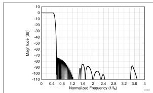
Figure 6-27. Linear Phase Decimation Filter
