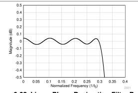
Figure 6-32. Linear Phase Decimation Filter Pass-**Band Ripple**
