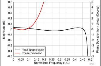
Figure 6-59. Ultra-Low-Latency Decimation Filter Magnitude Response
