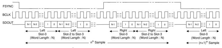
Figure 6-5. I<sup>2</sup>S Mode Standard Protocol Timing (TX OFFSET = 0)
