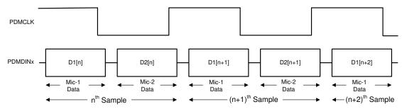
Figure 6-15. Digital PDM Microphone Protocol Timing Diagram
