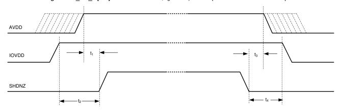
Figure 9-1. Power-Supply Sequencing Requirement Timing Diagram
