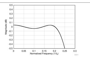
Figure 6-34. Linear Phase Decimation Filter Pass-Band Ripple
