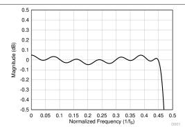
Figure 6-24. Linear Phase Decimation Filter Pass-**Band Ripple**
