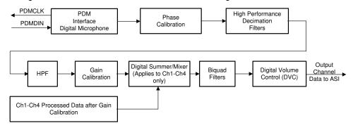
Figure 6-16. Signal-Chain Processing Flowchart
