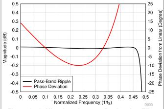
Figure 6-51. Ultra-Low-Latency Decimation Filter Magnitude Response
