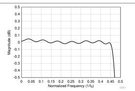
Figure 6-20. Linear Phase Decimation Filter Pass-Band Ripple
