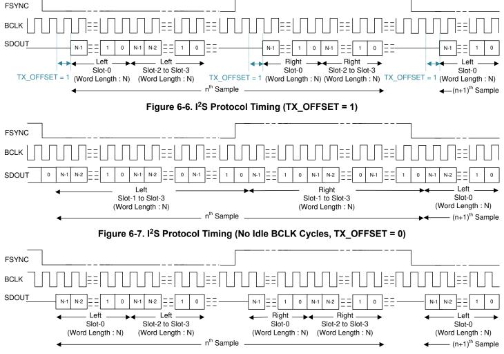
Figure 6-8. I<sup>2</sup>S Protocol Timing (TX\_OFFSET = 0 and BCLK\_POL = 1)
