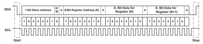
Figure 6-63. Typical I<sup>2</sup>C Sequence
