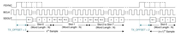
Figure 6-2. TDM Mode Protocol Timing (TX\_OFFSET = 2)
