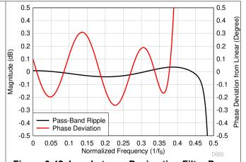
Figure 6-41. Low-Latency Decimation Filter Magnitude Response
