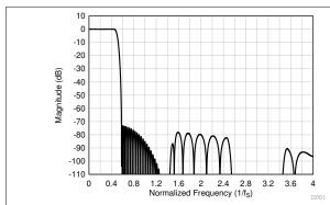
Figure 6-23. Linear Phase Decimation Filter Magnitude Response
