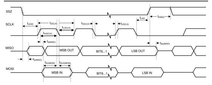
Figure 5-2. SPI Interface Timing Diagram
