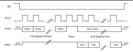
Figure 6-69. SPI Single-Byte Read Transfer
