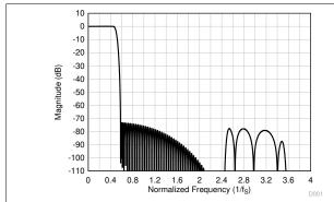
Figure 6-21. Linear Phase Decimation Filter Magnitude Response
