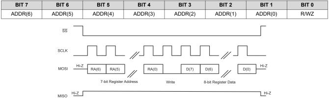
Figure 6-68. SPI Single-Byte Write Transfer
