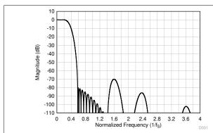
Figure 6-33. Linear Phase Decimation Filter Magnitude Response
