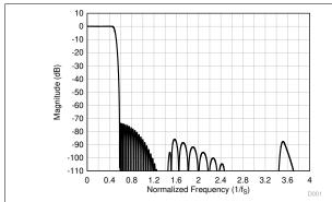
Figure 6-29. Linear Phase Decimation Filter Magnitude Response
