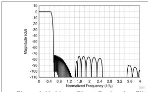
Figure 6-19. Linear Phase Decimation Filter Magnitude Response
