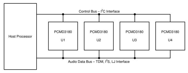
Figure 6-13. Multiple PCMD3180-Q1 Devices With Shared Control and Audio Data Buses
