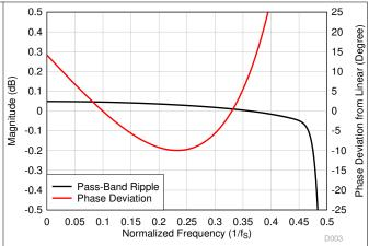
Figure 6-50. Ultra-Low-Latency Decimation Filter Pass-Band Ripple and Phase Deviation
