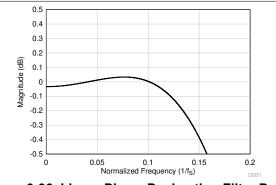
Figure 6-36. Linear Phase Decimation Filter Pass-Band Ripple
