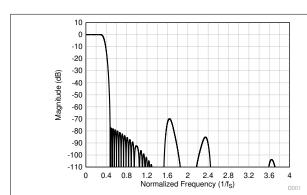
Figure 6-31. Linear Phase Decimation Filter Magnitude Response
