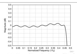
Figure 6-26. Linear Phase Decimation Filter Pass-Band Ripple
