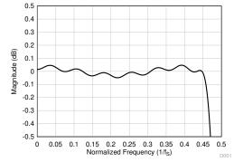
Figure 6-28. Linear Phase Decimation Filter Pass-Band Ripple
