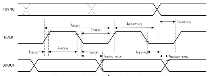
Figure 5-3. TDM (With BCLK\_POL = 1), I<sup>2</sup>S, and LJ Interface Timing Diagram
