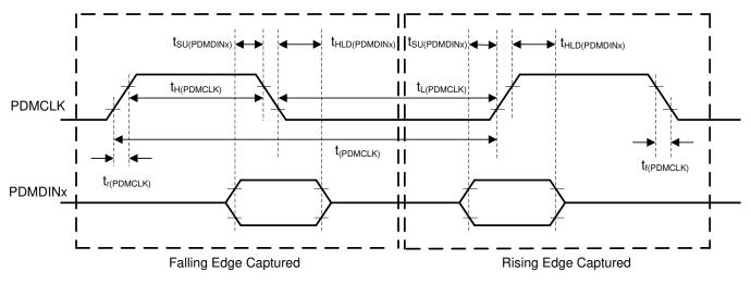
Figure 5-4. PDM Digital Microphone Interface Timing Diagram
