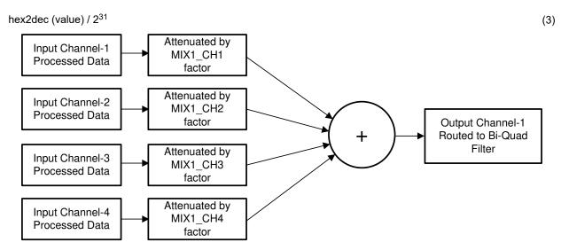
Figure 6-18. Programmable Digital Mixer Block Diagram
