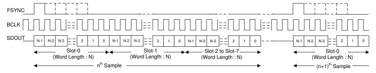
Figure 6-1. TDM Mode Standard Protocol Timing (TX OFFSET = 0)
