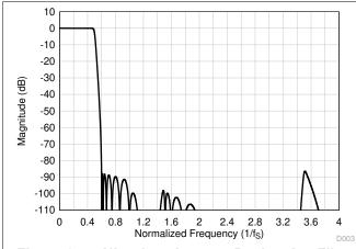
Figure 6-55. Ultra-Low-Latency Decimation Filter **Magnitude Response**
