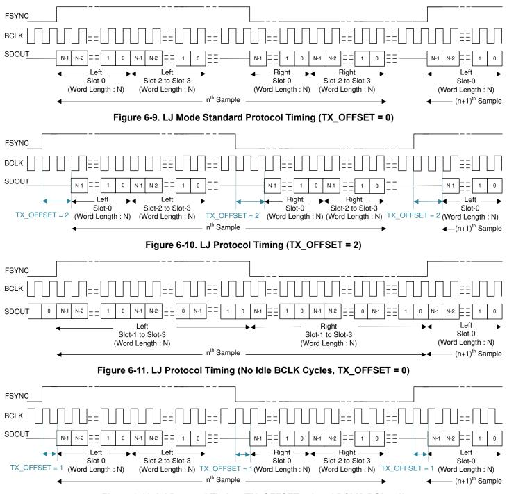
Figure 6-12. LJ Protocol Timing (TX\_OFFSET = 1 and BCLK\_POL = 1)
