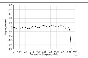
Figure 6-22. Linear Phase Decimation Filter Pass-**Band Ripple**
