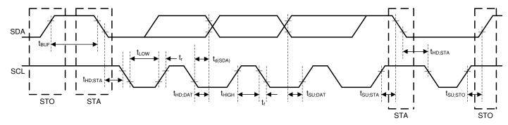
Figure 5-1. I<sup>2</sup>C Interface Timing Diagram
