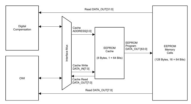
Figure 22. EEPROM Interface Structure
