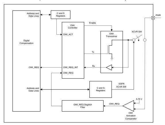
Figure 12. OWI System Components
