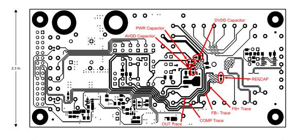
Figure 78. Layout Diagram
