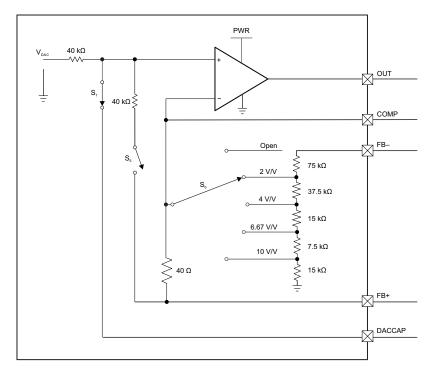
Figure 6. DAC Gain Stage Diagram
