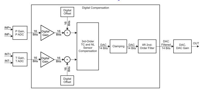
Figure 7. Digital Compensation and Filter Block Diagram
