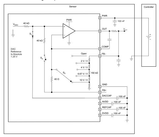
Figure 76. 0-V to 10-V Absolute Voltage Output Diagram
