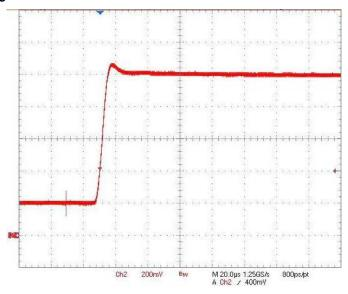
Figure 75. Loop Current Step From 4 mA to 20 mA
