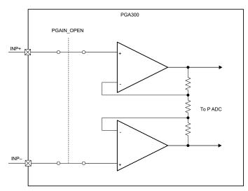
Figure 4. P Gain Stage Diagram
