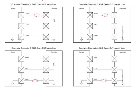
Figure 73. Harness Open-Wire Diagnostics
