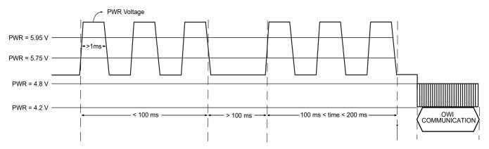
Figure 13. OWI Activation-Pulse Sequence Using Overvoltage Drive
