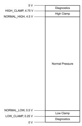
Figure 8. Example of Clamping the Digital Compensation Output
