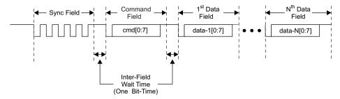
Figure 15. OWI Transmission Frame, N = 1 to 8
