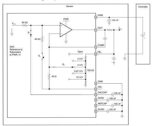
Figure 77. 0-V to 5-V Ratiometric Voltage Output Diagram
