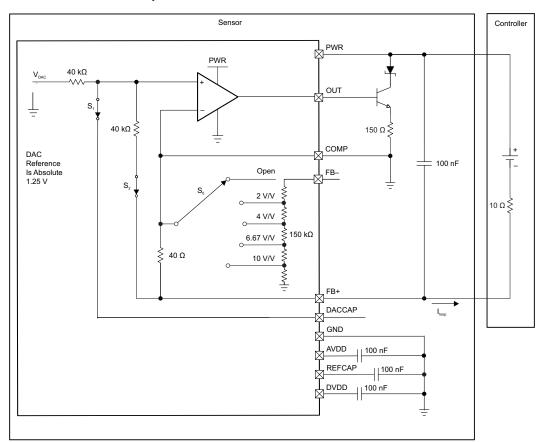
Figure 74. 4-mA to 20-mA Current Output Diagram
