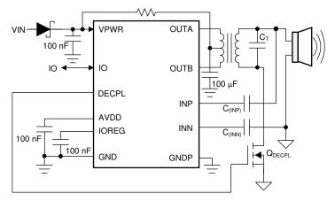
Figure 7-37. Transducer Time Decoupling
