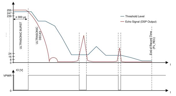
Figure 7-13. IO-Pin Object-Detection Signaling With Burst/Listen Time Command
