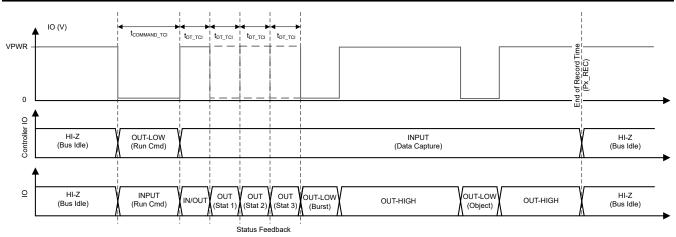
Figure 7-12. Time-Command Interface RUN Command Execution
