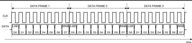
Figure 7-29. USART Synchronous Mode Data Flow
