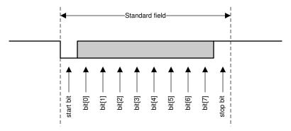
Figure 7-19. UART Interface Packet Field
