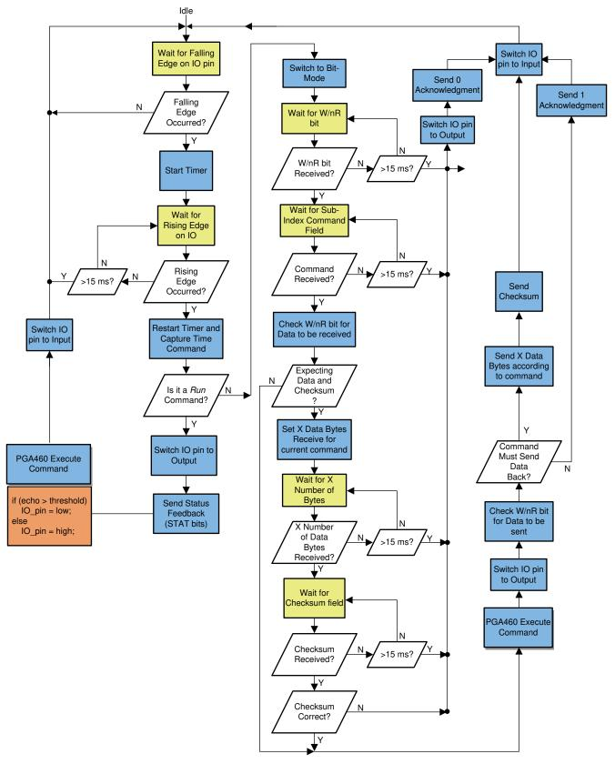
Figure 7-42. Time-Command Interface Communication Flow Chart
