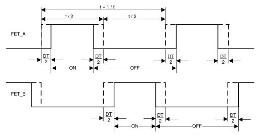
Figure 7-2. Echo Generation Dead-Time Adjustment
