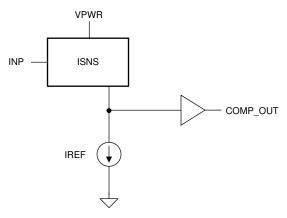
Figure 7-8. Block Diagram for Voltage Diagnostic
