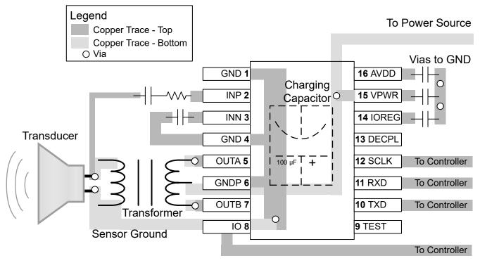
Figure 8-9. PGA460 Layout Example
