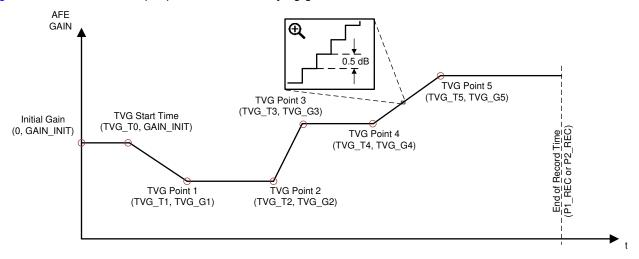
Figure 7-4. Time-Varying Gain Assignment Example
