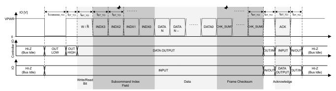
Figure 7-15. Time-Command Interface CONFIGURATION/STATUS Command—Write
