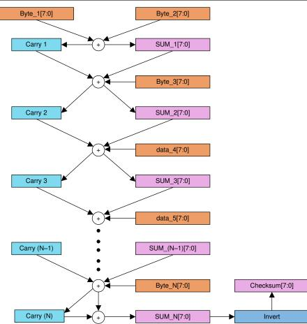
Figure 7-17. Checksum Calculation
