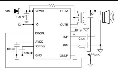
Figure 7-38. Transducer Temperature Decoupling
