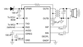
**Typical Application Diagram (Transformer Drive)**
