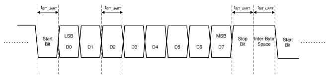
Figure 7-18. USART Asynchronous Interface Bit Timing
