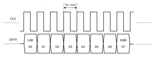
Figure 7-28. USART Synchronous Interface Bit Timing
