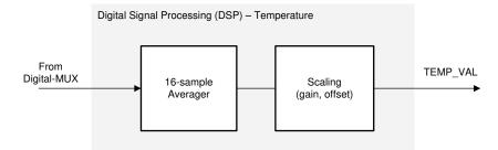
Figure 7-39. Temperature-Sensor Signal Path
