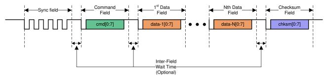
Figure 7-20. UART Interface Transmission Frame
