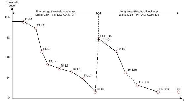
Figure 7-7. Example of DIG\_GAIN\_LR\_ST = [00] TH9
