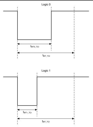
Figure 7-11. Time-Command Interface Bit Timing
