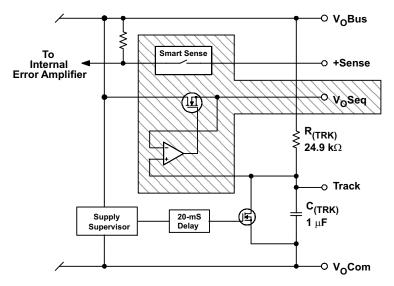
Note: The shaded functions are only available with the PTB48560B (3.3-V output).
