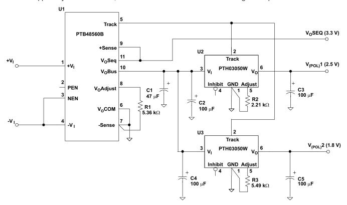
Figure 19. Power-Up Sequencing With Nonisolated POL Modules
