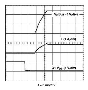
Figure 17. Output Enable Power-Up Characteristic
