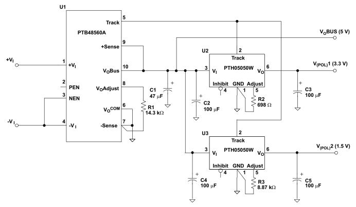
Figure 21. Power-Up Sequencing With Nonisolated POL Modules
