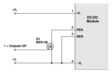
Figure 15. Positive Enable Configuration
