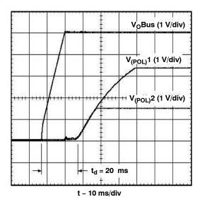
Figure 22. Power-Up Waveform
