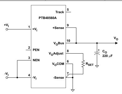
Figure 14. Output Voltage Adjustment
