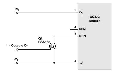
Figure 16. Negative Enable Configuration
