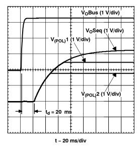
Figure 20. Power-Up Waveforms with POL Modules
