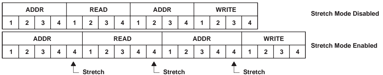
Figure 8. One 32-Bit Nonpage-Mode Read-Write
