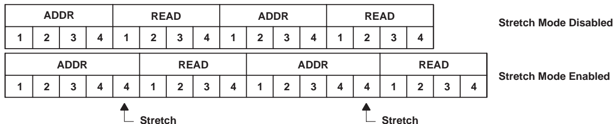
Figure 5. Two 32-Bit Nonpage-Mode Reads
