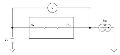
Figure 7-1. On-Resistance Measurement Setup
