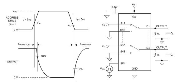
Figure 7-5. Transition-Time Measurement Setup
