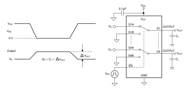
Figure 7-11. Charge-Injection Measurement Setup
