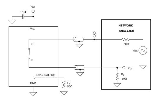
Figure 7-15. Bandwidth Measurement Setup
