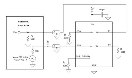
Figure 7-14. Channel-to-Channel Crosstalk Measurement Setup
