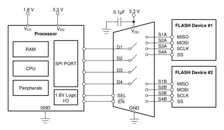
Figure 9-1. Multiplexing Flash Memory
