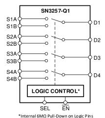
Figure 8-1. SN3257-Q1 Functional Block Diagram
