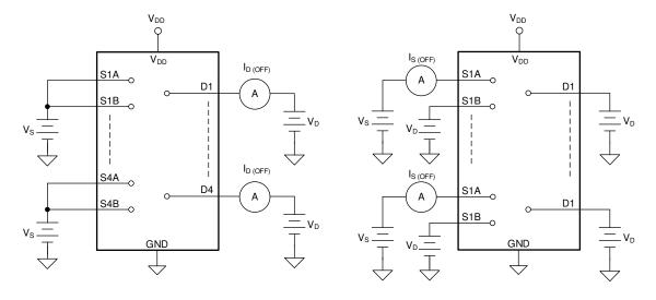
Figure 7-2. Off-Leakage Measurement Setup
