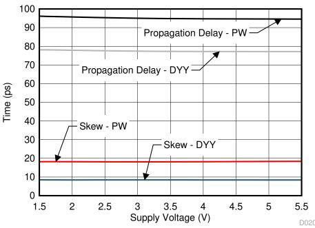
Figure 9-2. Propagation Delay and Skew Measurement
