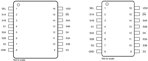
Figure 5-1. PW Package, 16-Pin TSSOP (Top View)
