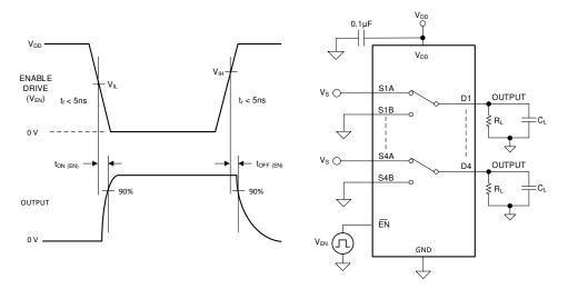
Figure 7-6. t<sub>ON (EN)</sub> and t<sub>OFF (EN)</sub> Time Measurement Setup
