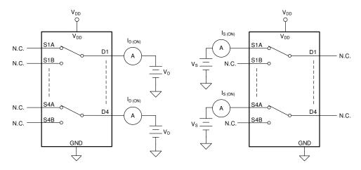
Figure 7-3. On-Leakage Measurement Setup
