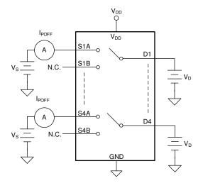
Figure 7-4. I<sub>POFF</sub> Leakage Measurement Setup
