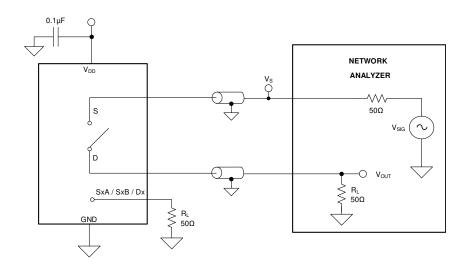
Figure 7-13. Off Isolation Measurement Setup
