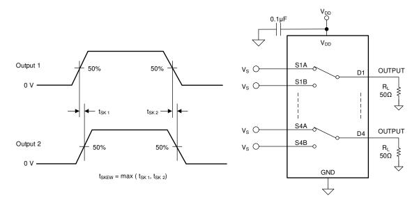
Figure 7-10. Skew Measurement Setup
