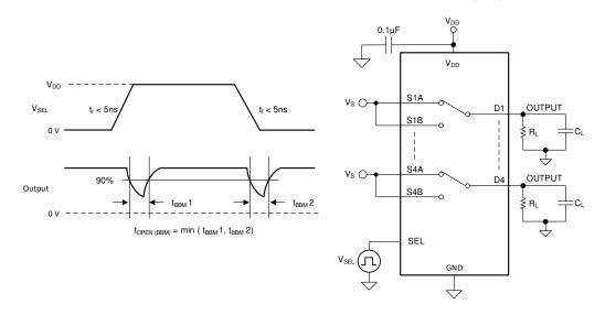
Figure 7-8. Break-Before-Make Delay Measurement Setup
