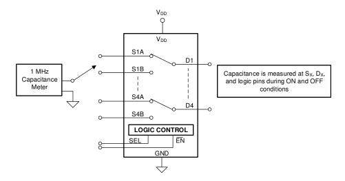
Figure 7-12. Capacitance Measurement Setup
