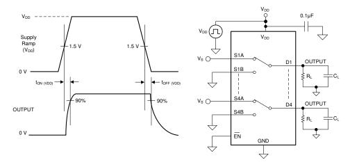
Figure 7-7. t<sub>ON (VDD)</sub> and t<sub>OFF (VDD)</sub> Time Measurement Setup
