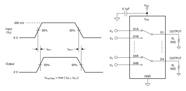
Figure 7-9. Propagation Delay Measurement Setup
