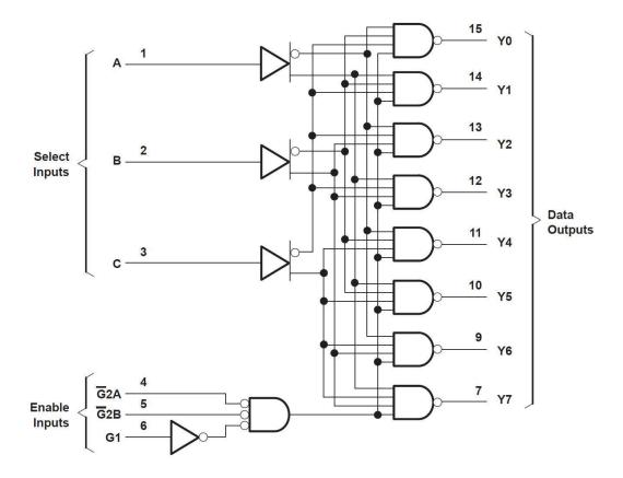
Figure 6-1. Logic Diagram (Positive Logic)
