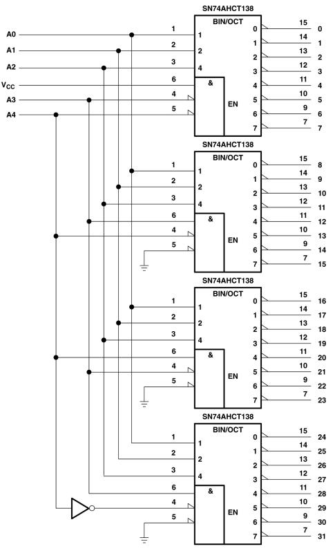
Figure 7-2. 32-Bit Decoding Scheme
