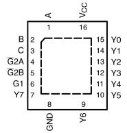
Figure 3-1. SN54AHCT138 J or W Package; SN74AHCT138 D, DB, DGV, N, NS, or PW Package (Top View)
