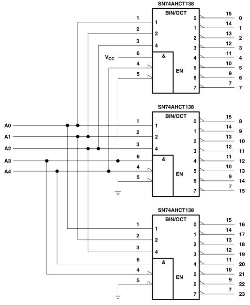
Figure 7-1. 24-Bit Decoding Scheme
