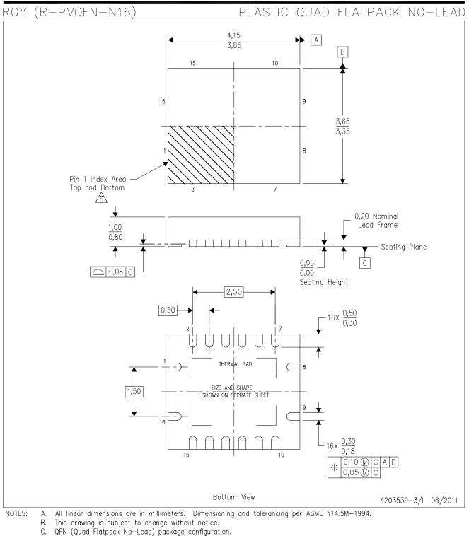
D. The package thermal pad must be soldered to the board for thermal and mechanical performance.
