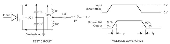
A. C1, C2, and C3 include probe and jig capacitance.
