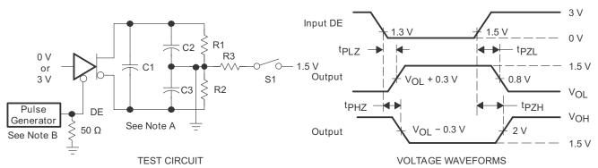
A. C1, C2, and C3 include probe and jig capacitance.
