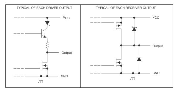
Figure 7-2. Schematic of Outputs
