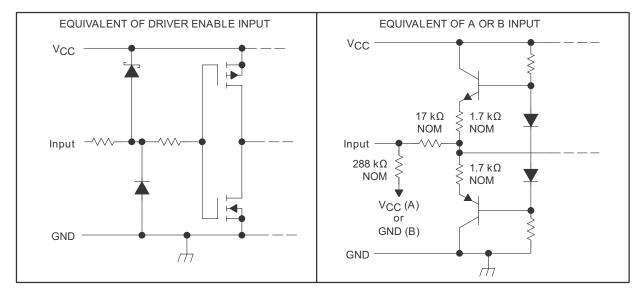
Figure 7-1. Schematic of Inputs
