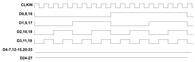
The 16 grayscale test pattern test device power consumption for a typical display pattern.
