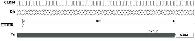
Figure 12. Enable Time Waveforms
