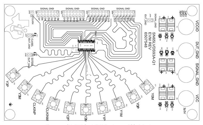
Figure 24. SN65LVDS93A EVM Top Layer - TSSOP Package
