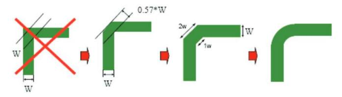
Figure 23. Poor and Good Right-Angle Bends
