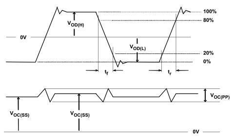
Figure 7. Test Load and Voltage Definitions for LVDS Outputs
