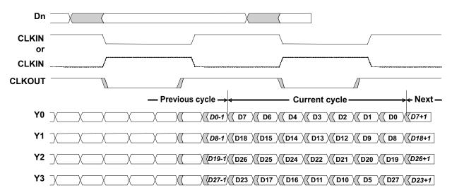
Figure 1. Typical SN65LVDS93A Load and Shift Sequences
