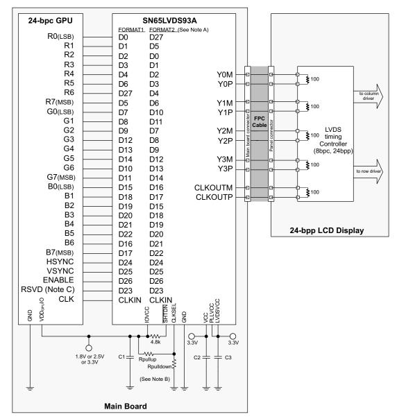
Note A. **FORMAT**: The majority of 24-bit LCD display panels require the two most significant bits (2 MSB) of each color to be transferred over the 4th serial data output Y3. A few 24-bit LCD display panels require the two LSBs of each color to be transmitted over the Y3 output. The system designer needs to verify which format is expected by checking the LCD display data sheet.
