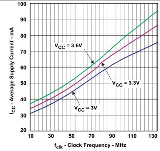
Total device current (using grayscale pattern) over pixel clock frequency
