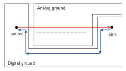
Figure 21. Loop Area and Crosstalk Due to Poor Signal Routing and Ground Splitting
