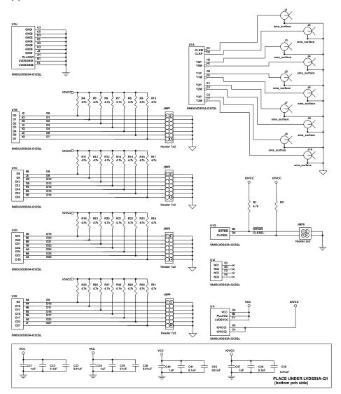
Figure 14. Schematic Example (SN65LVDS93A Evaluation Board)
