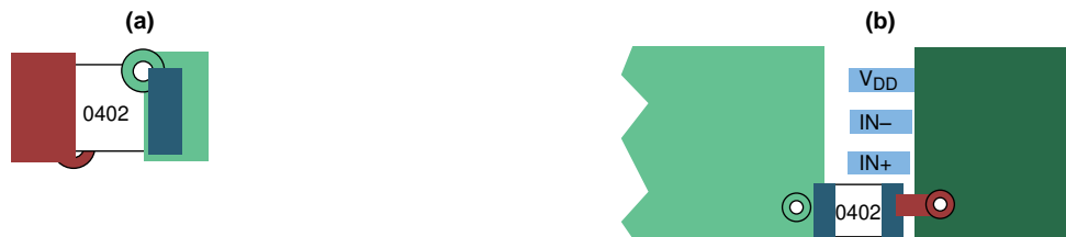
Figure 28. Typical Decoupling Capacitor Layouts
