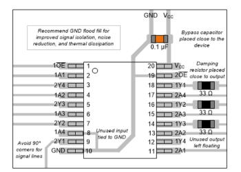
Figure 8-1. Layout Example for the SNx4AC244 in the PW Package
