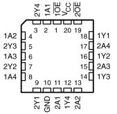
Figure 4-3. SN54AC244 FK Package (Top View)
