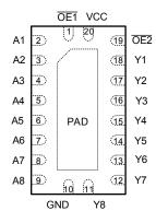
Figure 4-2. RKS Package, 20-Pin VQFN (Top View)
