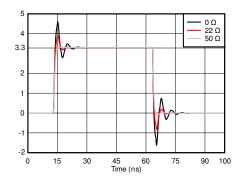
Figure 8-2. Simulated Signal Integrity at the Receiver with Different Damping Resistor (R<sub>d</sub>) Values
