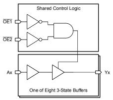
Logic Diagram (Positive Logic)
