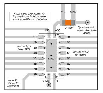
Figure 7-3. Example Layout for the SN74AC573-Q1 in the RKS Package
