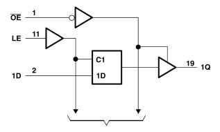
To Seven Other Channels Figure 6-1. Logic Diagram (Positive Logic)
