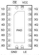
Figure 4-1. SN74AC573-Q1 PW Package, 20-Pin TSSOP (Top View)
