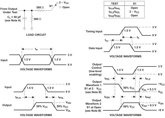
A. C<sub>L</sub> includes probe and jig capacitance.
