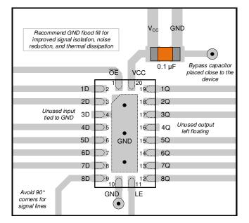
Figure 7-3. Example Layout for the SN74ACT573-Q1 in the RKS Package
