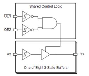
Figure 6-1. Logic Diagram (Positive Logic)
