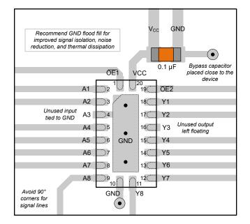
Figure 7-3. Example Layout for the SN74ACT8541 in the RKS Package
