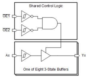
Logic Diagram (Positive Logic)
