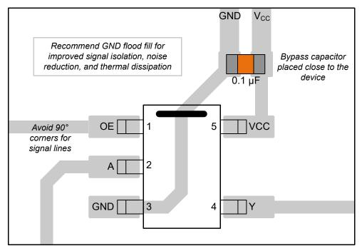
Figure 9-3. Example Layout for the SN74AHCT1G126-Q1
