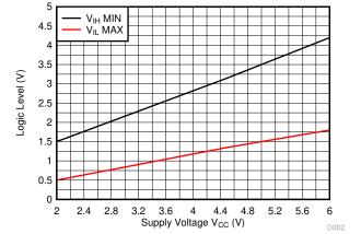
Figure 9-2. Input High and Input Low Thresholds vs Supply Voltage
