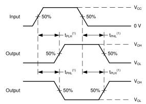
A. The maximum between t<sub>PLH</sub> and T<sub>PHL</sub> is used for t<sub>pd</sub>.
