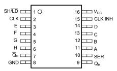
Figure 5-1. SN74HC165B-EP: PW Package, 16-Pin TSSOP (Top View)
