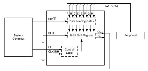
Figure 9-1. Input Expansion with Shift Registers
