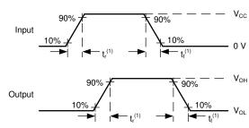
A. The maximum between  $t_r$  and  $t_f$  is used for  $t_t$ .
