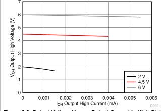
Figure 6-3. Output Voltage Versus Output Current in High State
