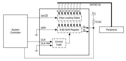
Figure 9-1. Typical application block diagram
