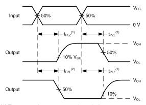
(1) The greater between  $t_{\text{PLZ}}$  and  $t_{\text{PZL}}$  is the same as  $t_{\text{pd}}$ .
