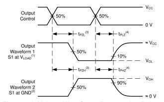
Figure 7-3. Voltage Waveforms Propagation Delays
