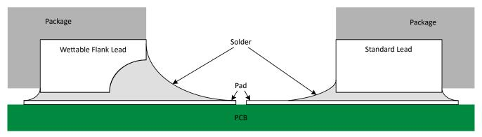
Figure 8-3. Simplified Cutaway View of Wettable-Flank QFN Package and Standard QFN Package After Soldering
