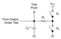
(1) C<sub>L</sub> includes probe and test-fixture capacitance.
