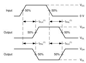
(1) The greater between  $t_{PLH}$  and  $t_{PHL}$  is the same as  $t_{pd}$ .
