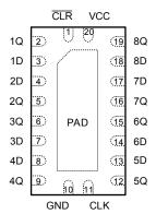
RKS Package 20-Pin VQFN (Top View)
