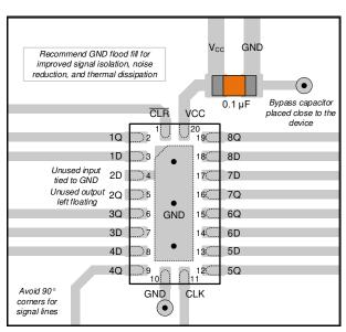
Figure 11-2. Example Layout for the SN74HCS273 RKS Package
