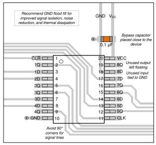
Figure 11-1. Example Layout for the SN74HCS273 PW Package
