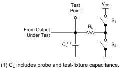
Figure 7-1. Load Circuit for 3-State Outputs
