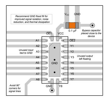
Figure 11-1. Example Layout for the SN74HCS541 in the RKS Package
