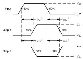
(1) The greater between t<sub>PLH</sub> and t<sub>PHL</sub> is the same as t<sub>pd</sub>. **Figure 7-2. Voltage Waveforms Propagation Delays**
