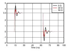
Figure 9-2. Simulated Signal Integrity at the Receiver With Different Damping Resistor (R<sub>d</sub>) Values
