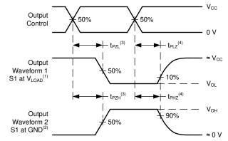
Figure 7-3. Voltage Waveforms Propagation Delays
