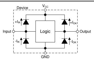
Figure 8-2. Electrical Placement of Clamping Diodes for Each Input and Output
