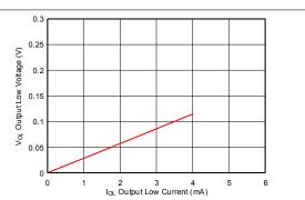
Figure 6-1. Typical Output Voltage in the High State | Figure 6-2. Typical Output Voltage in the Low State (V<sub>OL</sub>)
