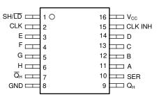
Figure 5-1. PW Package 16-Pin TSSOP Top View
