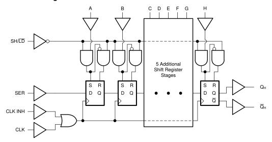
Figure 8-1. Logic Diagram (Positive Logic) for SN74HCT165
