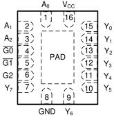
Figure 5-1. BQB Package 16-Pin (Top View)
