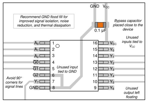
Figure 11-1. Layout Example for the SN74LV138A-Q1
