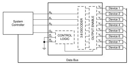
Figure 9-1. Output Exapnsion with Multiplexer
