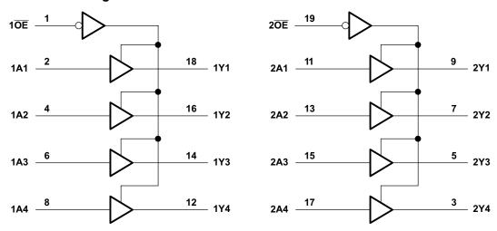
Figure 8-1. Logic Diagram (Positive Logic)
