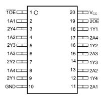
Figure 5-2. SN74LV244A-Q1: DGS Package, 20-Pin VSSOP (Top View)
