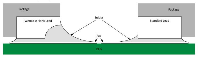
Figure 8-2. Simplified Cutaway View of Wettable-Flank QFN Package and Standard QFN Package After Soldering
