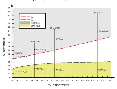
Figure 8-2. LVxT Input Voltage Levels
