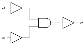
Simplified Logic Diagram (Positive Logic)
