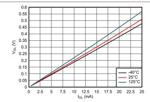
Figure 6-9. Output Voltage vs Current in LOW State; 3.3-V Supply
