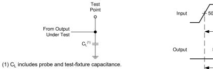
Figure 7-1. Load Circuit for Push-Pull Outputs
