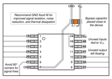
Figure 11-1. Example Layout for the SN74LV4T08
