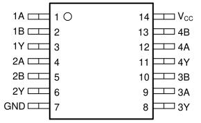
Figure 5-2. PW Package, 14-Pin TSSOP (Top View)
