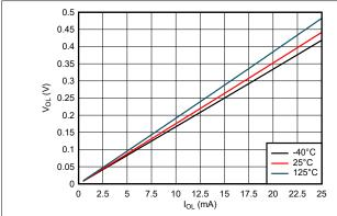
Figure 6-7. Output Voltage vs Current in LOW State; 5-V Supply
