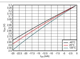
Figure 6-8. Output Voltage vs Current in HIGH State; 3.3-V Supply
