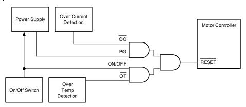
Figure 9-1. Typical Application Block Diagram
