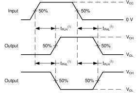
(1) The greater between t<sub>PLH</sub> and t<sub>PHL</sub> is the same as t<sub>pd</sub>. Figure 7-2. Voltage Waveforms Propagation Delays
