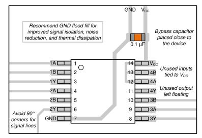
Figure 9-3. Example Layout for the SN74LV4T32
