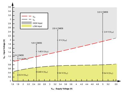
Figure 8-2. LVxT Input Voltage Levels
