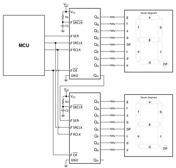
Figure 9-1. Input Expansion with Shift Registers
