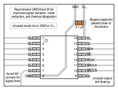
Figure 9-3. Layout Example for the SN74LV595B-EP in the PW Package
