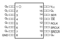
Figure 5-1. SN74LV595B-EP: PW Package, 16-Pin TSSOP (Top View)
