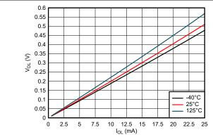
Figure 6-9. Output Voltage vs Current in LOW State; 3.3-V Supply
