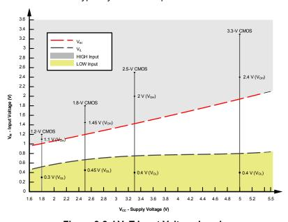
Figure 8-2. LVxT Input Voltage Levels
