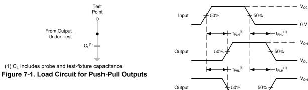
(1) The greater between  $t_{\text{PLH}}$  and  $t_{\text{PHL}}$  is the same as  $t_{\text{pd}}$ .
