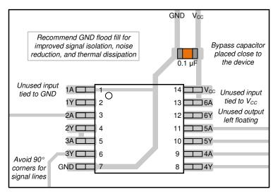
Figure 11-1. Example Layout for the SN74LV6T14
