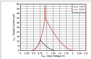
Figure 6-1. Supply Current Across Input Voltage 1.8-V and 2.5-V | Figure 6-2. Supply Current Across Input Voltage 3.3-V and 5.0-V Supply
