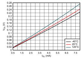
Figure 6-13. Output Voltage vs Current in LOW State; 1.8-V Supply
