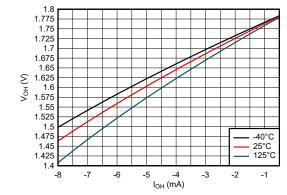
Figure 6-12. Output Voltage vs Current in HIGH State; 1.8-V Supply
