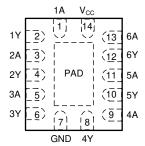
Figure 5-1. SN74LV6T14 BQA Package, 14-Pin WQFN (Top View)
