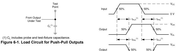
(1) The greater between  $t_{PLH}$  and  $t_{PHL}$  is the same as  $t_{pd}$ .
