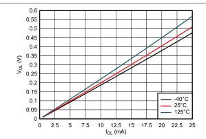
Figure 5-9. Output Voltage vs Current in LOW State; 3.3V Supply
