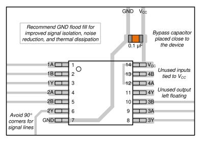
Figure 10-1. Example Layout for the SN74LV6T17-EP
