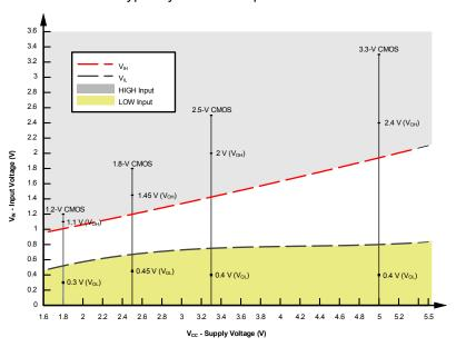
Figure 7-2. LVxT Input Voltage Levels
