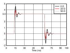
Figure 8-2. Simulated Signal Integrity at the Receiver With Different Damping Resistor (R<sub>d</sub>) Values
