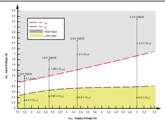
Figure 7-3. LVxT Input Voltage Levels
