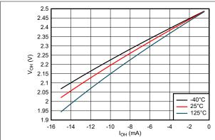
Figure 5-7. Output Voltage vs Current in HIGH State; 2.5V Supply
