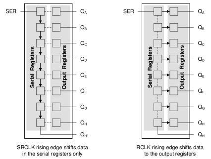
Figure 8-2. Simplified Functional Diagram Showing Clock Operation
