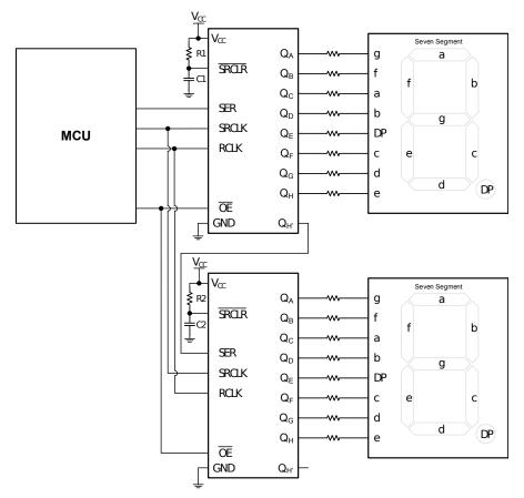
Figure 8-1. Typical Application Block Diagram
