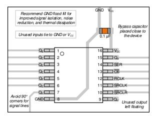
Figure 8-3. Example Layout for the SN74LV8T596 in TSSOP
