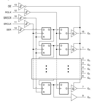
Figure 7-1. Logic Diagram (Positive Logic) for SN74LV8T596
