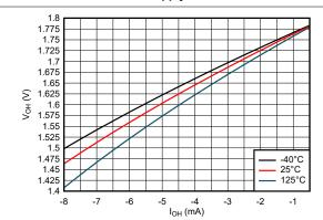
Figure 5-9. Output Voltage vs Current in HIGH State; 1.8V
