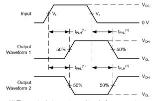
(1) The greater between  $t_{PLH}$  and  $t_{PHL}$  is the same as  $t_{pd}$ . Figure 6-2. Voltage Waveforms Propagation Delays
