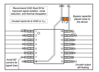
Figure 8-3. Example Layout for the SN74LVC2G100
