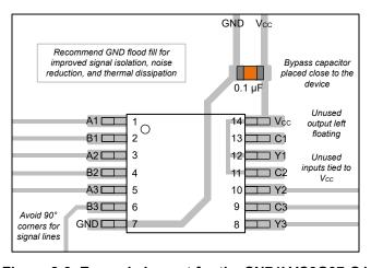
Figure 8-3. Example Layout for the SN74LVC3G97-Q1
