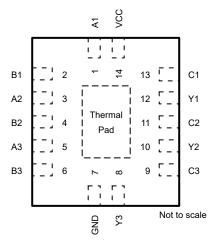
Figure 4-1. SN74LVC3G97-Q1 PW Package (Preview), 14-Pin TSSOP (Top View)
