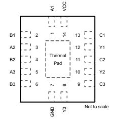
Figure 4-2. SN74LVC3G98 BQA Package, 14-Pin WQFN (Top View)
