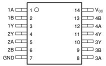
Figure 4-2. SN74LVC7266A-Q1 PW Package, 14-Pin TSSOP (Top View)
