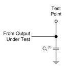
(1) C<sub>L</sub> includes probe and test-fixture capacitance.
