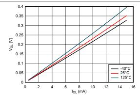
Figure 5-11. Output Voltage vs Current in LOW State; 2.5V
