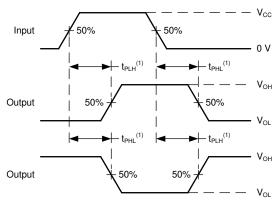
(1) The greater between  $t_{\text{PLH}}$  and  $t_{\text{PHL}}$  is the same as  $t_{\text{pd}}.$
