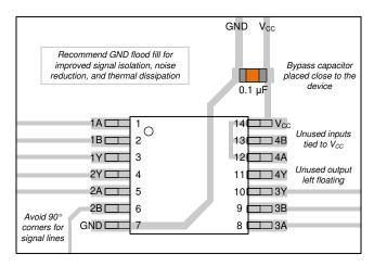
Figure 8-3. Example Layout for the SN74LVC7266A-Q1
