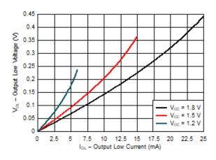
Figure 6-4. Typical ( $T_A$ =25°C) Output High Voltage ( $V_{OL}$ ) vs Sink Current ( $I_{OL}$ )
