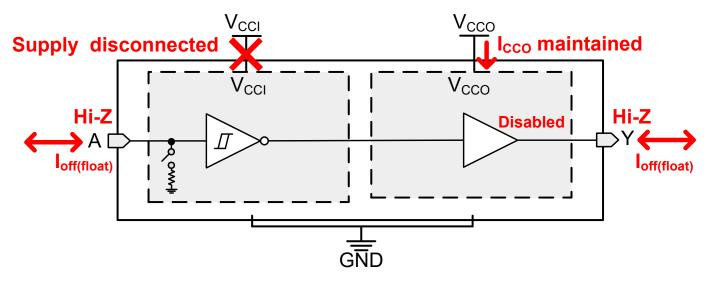
Figure 8-1. V<sub>CC</sub> Disconnect Feature
