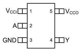
Figure 5-1. DCK Package, 5-Pin SC70 (Top View)
