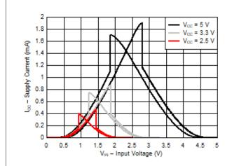
Figure 6-5. Typical (T\_A=25°C) Supply Current (I\_CC) vs Input Voltage (V\_IN)
