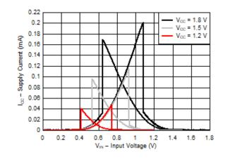
Figure 6-6. Typical (T<sub>A</sub>=25°C) Supply Current (I<sub>CC</sub>) vs Input Voltage (V<sub>IN</sub>)
