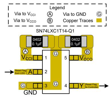
Figure 11-1. Layout Example - SN74LXC1T14-Q1
