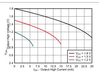
Figure 6-2. Typical (T<sub>A</sub>=25°C) Output High Voltage (V<sub>OH</sub>) vs Source Current (I<sub>OH</sub>)
