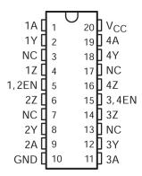
Figure 4-2. DW Package (Top View)
