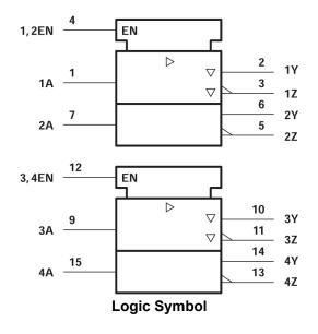
the requirements of ANSI Standards EIA/TIA-422-B and RS-485 and ITU Recommendation V.11. The device is optimized for balanced multipoint bus transmission at rates up to 4 megabaud. Each driver features wide positive and negative common-mode output voltage ranges making it suitable for party-line applications in noisy environments.
