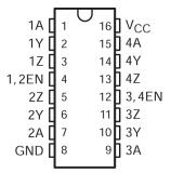
Figure 4-1. N Package (Top View)
