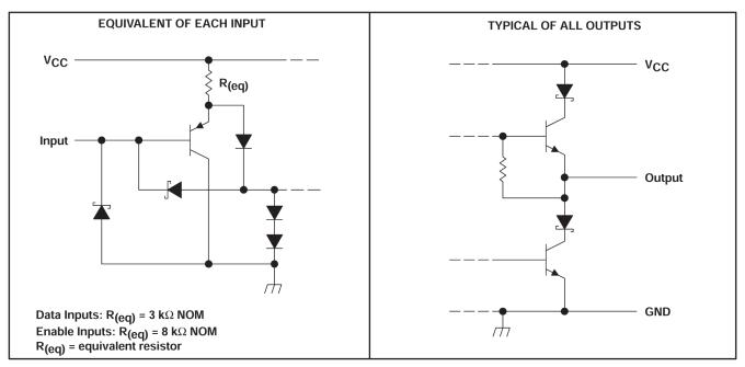
Figure 7-1. Schematics of Inputs and Outputs
