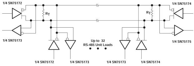
A. The line length should be terminated at both ends in its characteristic impedance (R<sub>T</sub> = Z<sub>O</sub>). Stub lengths off the main line should be kept as short as possible.
