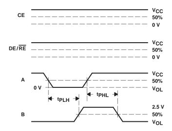
NOTES: A. All input pulses are supplied by a generator having the following characteristics:  $t_f \le 6$  ns,  $t_f \le 6$  ns, PRR  $\le 1$  MHz, duty cycle = 50%,  $Z_O = 50$   $\Omega$ .
