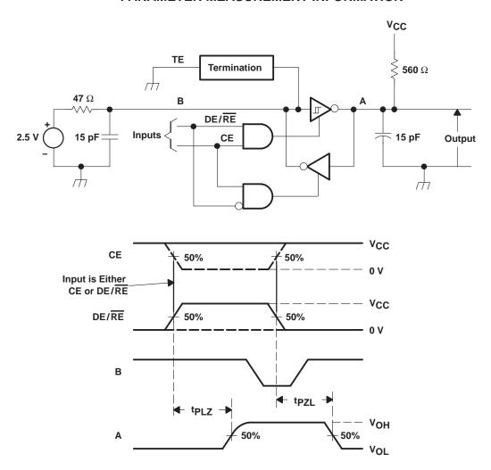
NOTES: A. All input pulses are supplied by a generator having the following characteristics:  $t_{\text{f}} \leq 6$  ns,  $t_{\text{f}} \leq 6$  ns, PRR  $\leq 1$  MHz, duty cycle = 50%,  $Z_{\text{O}} = 50~\Omega$ .
