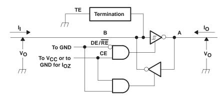
Figure 3. Receiver Voltages, Currents, and Test Circuit
