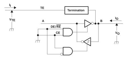
Figure 2. Active Termination Voltages, Currents, and Test Circuit.
