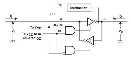
Figure 1. Driver Test Circuit Currents and Voltages.
