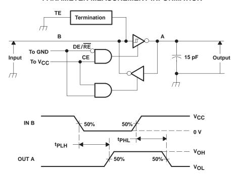
NOTES: A. All input pulses are supplied by a generator having the following characteristics:  $t_{\Gamma} \leq$  6 ns,  $t_{f} \leq$  6 ns, PRR  $\leq$  1 MHz, duty cycle = 50%,  $Z_{O}$  = 50  $\Omega$ .
