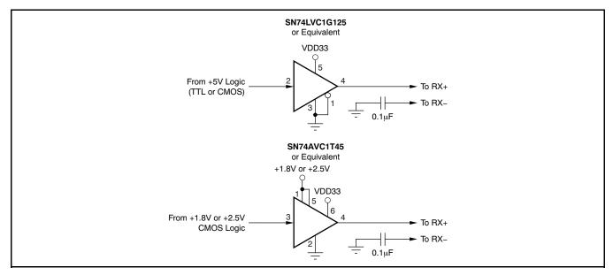
Figure 87. CMOS/TTL Input Logic Interface
