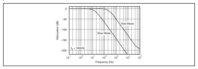
Figure 73. Input Digital Servo-Loop Frequency Response
