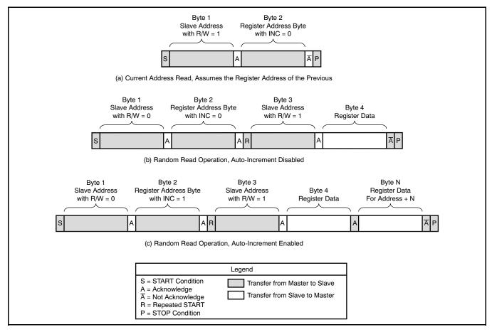
Figure 78. Fast/Standard Mode Read Operations
