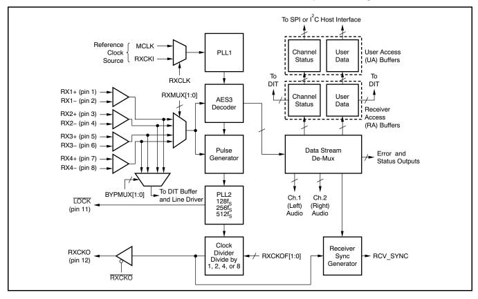
Figure 67. Digital Interface Receiver (DIR) Functional Block Diagram
