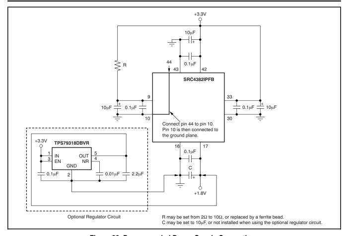
Figure 82. Recommended Power-Supply Connections
