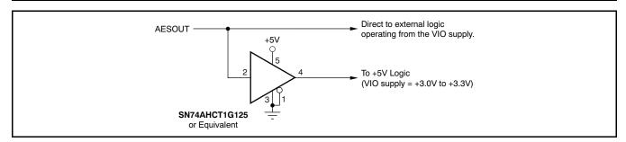
Figure 91. CMOS/TTL Output Logic Interface
