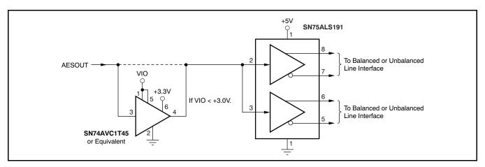
Figure 92. External Line Driver Interface
