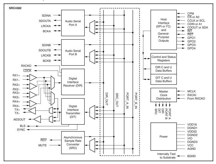
Figure 59. Functional Block Diagram
