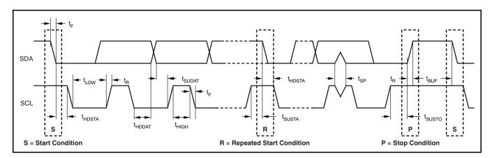
Figure 3. I<sup>2</sup>C Standard and Fast Mode Timing
