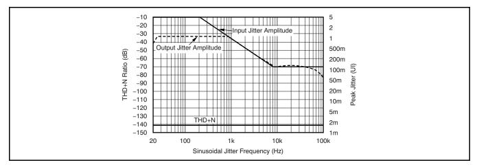
Figure 70. DIR Jitter Tolerance Plot
