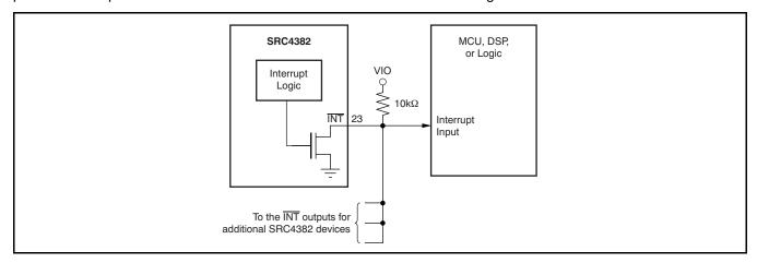
Figure 79. Interrupt Output Pin Connections
