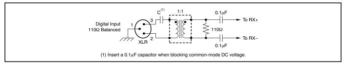
Figure 83. Transformer-Coupled Balanced Input Interface
