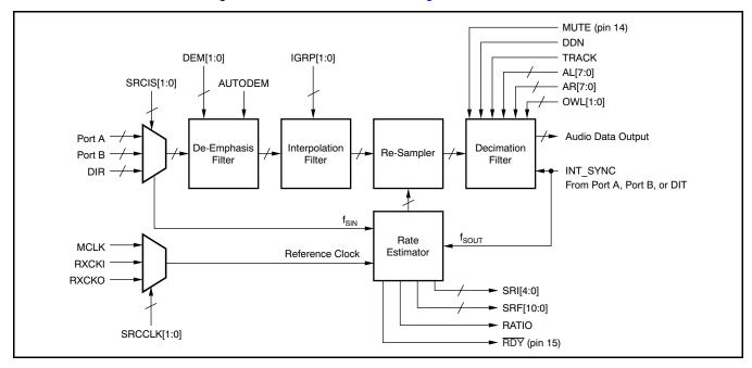
Figure 72. Asynchronous Sample Rate Converter (SRC) Functional Block Diagram
