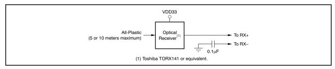
Figure 85. Interfacing to a +3.3V Optical Receiver Module
