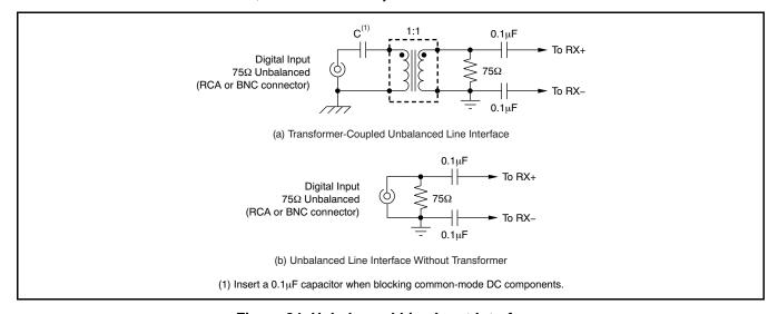
Figure 84. Unbalanced Line Input Interfaces
