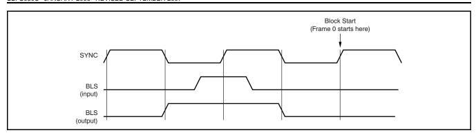
Figure 66. DIT Block Start Timing
