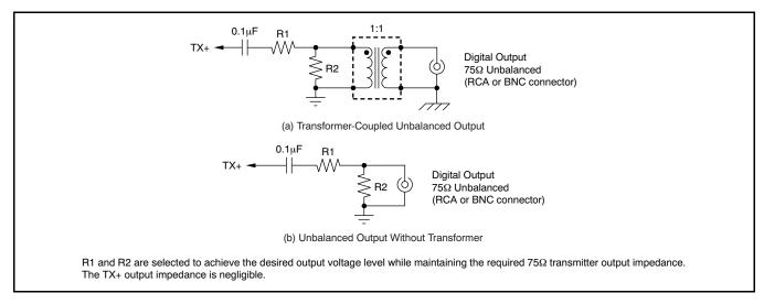
Figure 89. Unbalanced Line Output Interfaces
