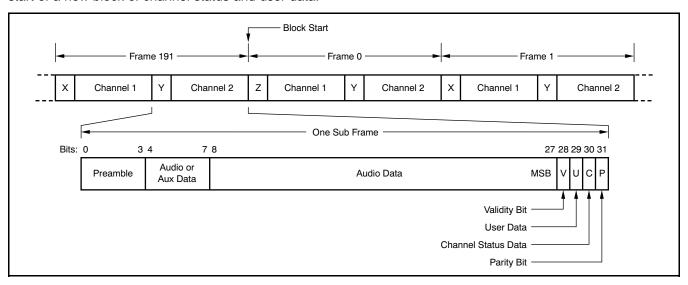
Figure 63. AES3 Frame and Subframe Encoding
