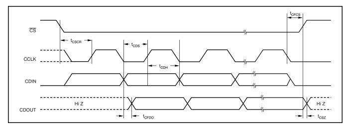
Figure 2. SPI Interface Timing
