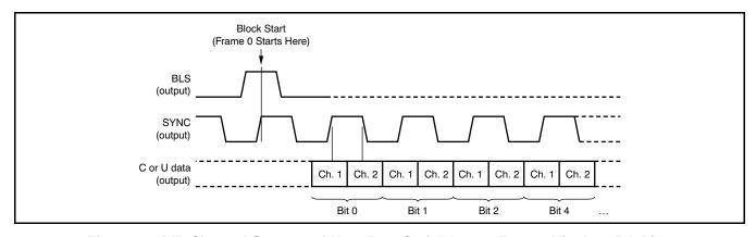
Figure 71. DIR Channel Status and User Data Serial Output Format Via the GPO Pins
