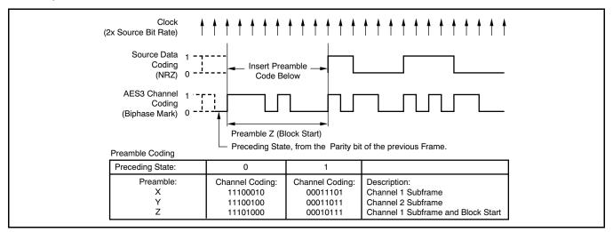
Figure 64. Biphase Mark Encoding
