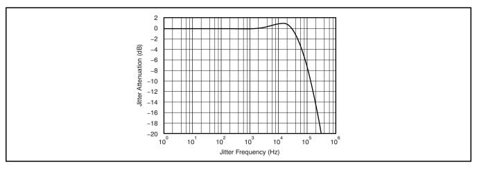
Figure 69. DIR Jitter Attenuation Characteristics
