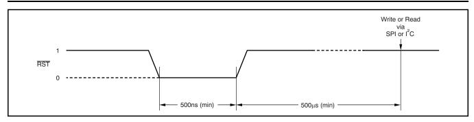
Figure 60. Reset Sequence Timing
