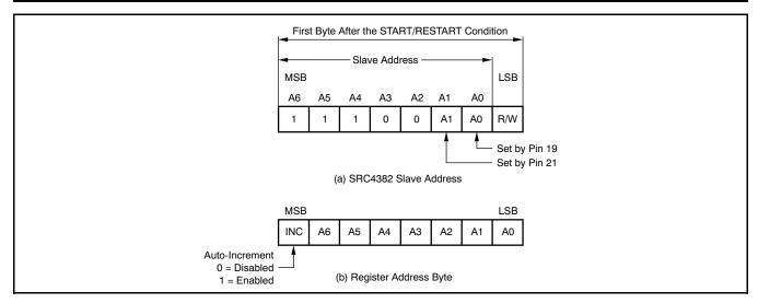
Figure 76. SRC4382 Slave Address and Register Address Byte Definitions
