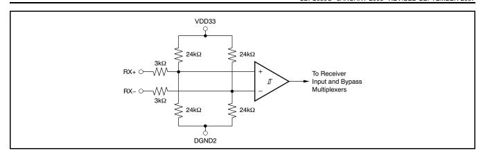
Figure 68. Differential Line Receiver Circuit
