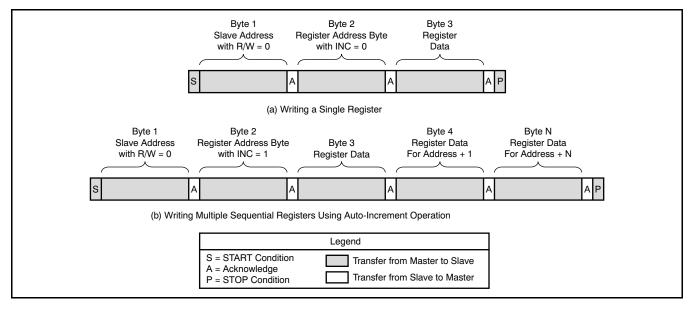
Figure 77. Fast/Standard Mode Write Operations
