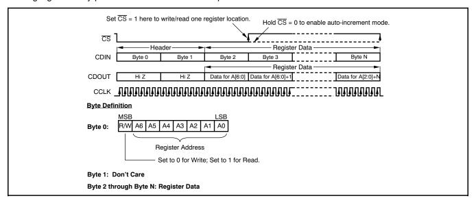
Figure 75. Serial Peripheral Interface (SPI) Protocol for the SRC4382
