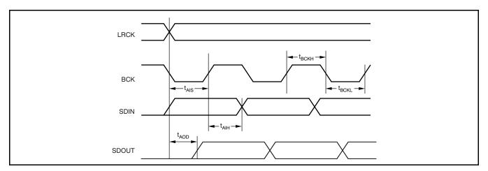
Figure 1. Audio Serial Port Timing
