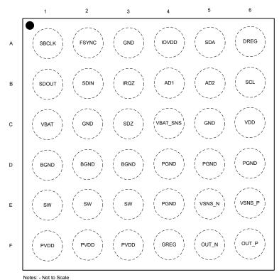
Figure 5-1. Package Top Level View Pinout
